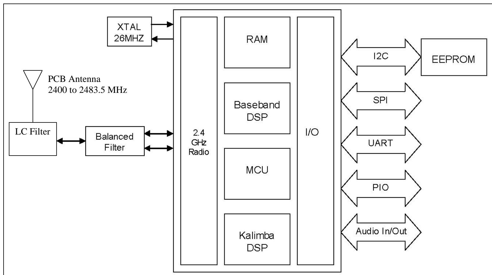
BC5MMRPA is a Class 2 Bluetooth sub-system using BlueCore5 –Multimedia ROM chipset from leading Bluetooth chipset supplier Cambridge Silicon Radio. It interfaces to a 32-kbit EEPROM using I2C interface. The software stack running on the BlueCore5 ROM chipset is fully compliant to Bluetooth Specification v2.1 + EDR. BC5MMRPA also has necessary balun and bandpass filters to interface with a build-in PCB antenna, which forms a very cost effective radio subsystem.
