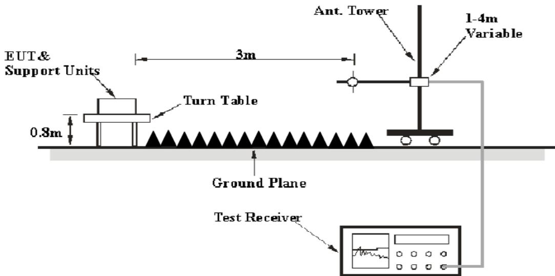
The radiated emission tests were performed in the 3 meters test site, using the setup accordance with the ANSI C63.4 - 2014. The specification used was the FCC 15§ 15.319(g).
