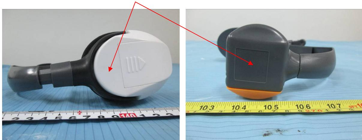
The label shown shall be permanently affixed at a conspicuous location on the device and be readily visible to the user at the time purchase (Labeling requirements per 2.925)
