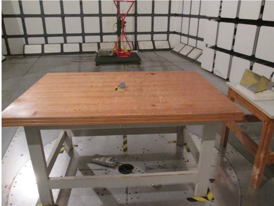
Radiated Emissions View (Below 1 GHz)
