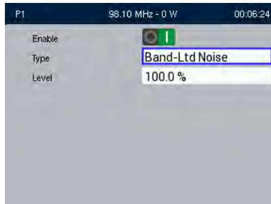
Figure 2.2.112: Signal Generator - Band Limited Noise
