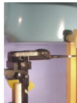
Face-held SAR Test Setup with 2.5cm spacing
