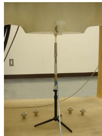
5100-5800MHz System performance check setup
