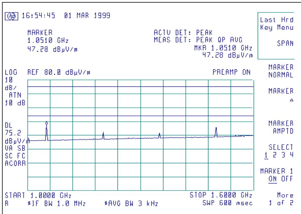
Radiated Emission signature scan, 162 MHz, horizontal polarity, 125 MW level
