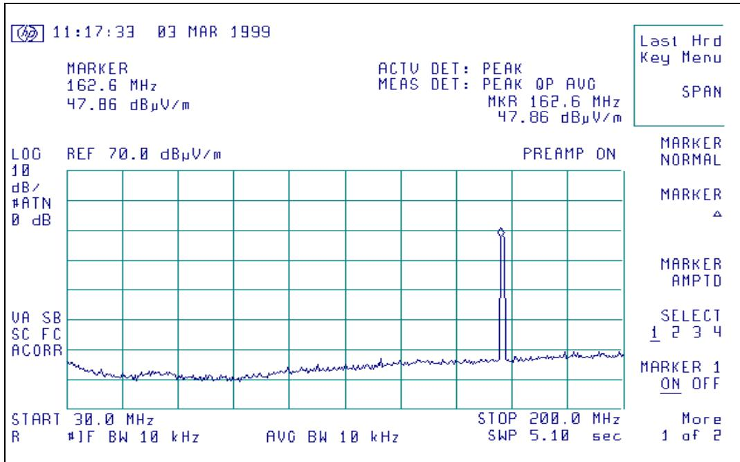
Radiated Emission signature scan, 174 MHz, vertical polarity, 125 MW level
