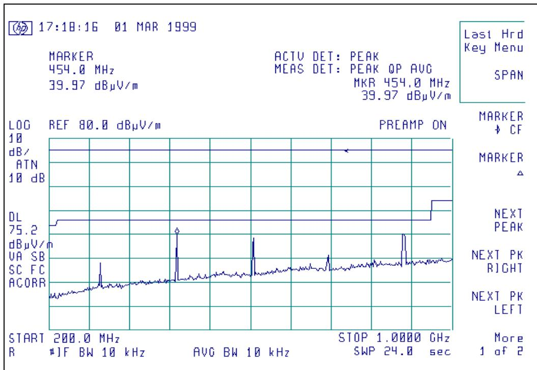
Radiated Emission signature scan, 150 MHz, vertical polarity, 50 MW level
