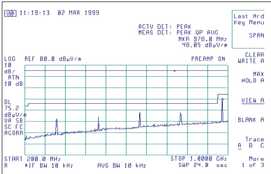
Radiated Emission signature scan, 162 MHz, vertical polarity, 125 MW level
