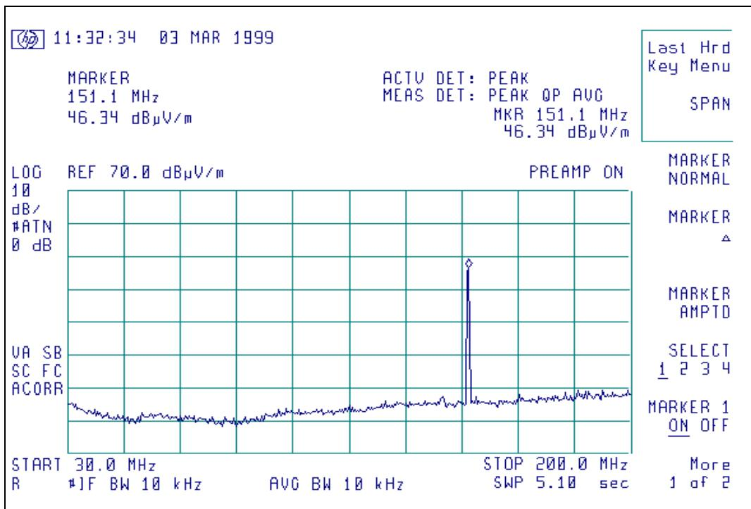
Radiated Emission signature scan, 150 MHz, horizontal polarity, 125 MW level
