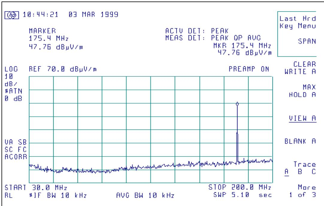
Radiated Emissions signature scan, 162 MHz, vertical polarity, 125 milliwatt level.
