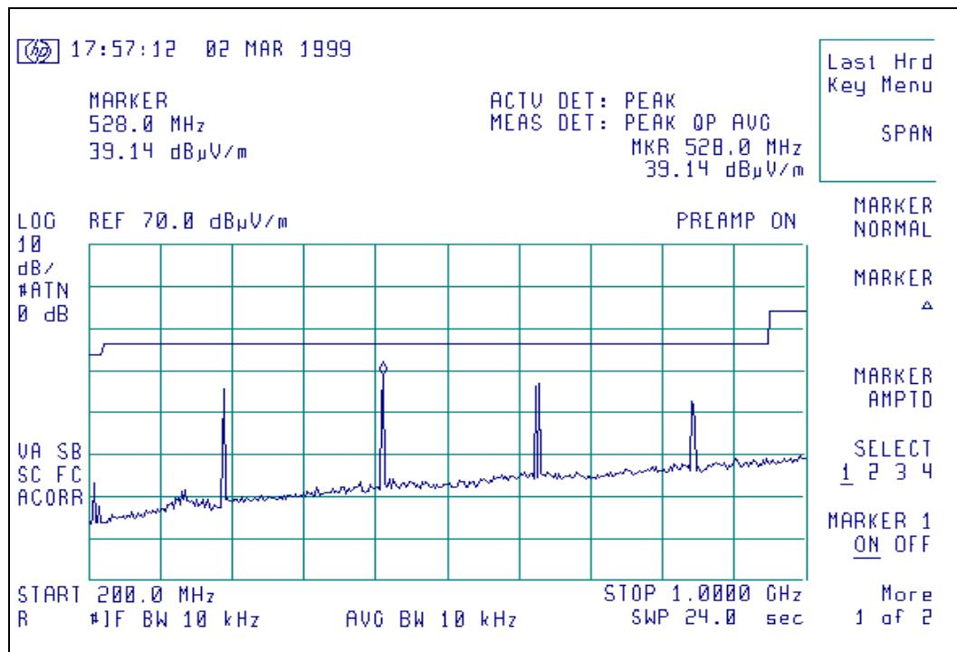
Radiated Emission signature scan, 174 MHz, vertical polarity, 50 MW level
