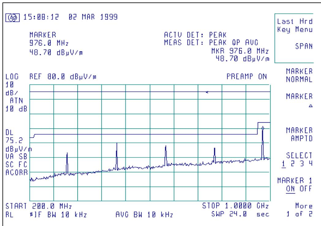
Radiated Emission signature scan, 162 MHz, vertical polarity, 50 MW level
