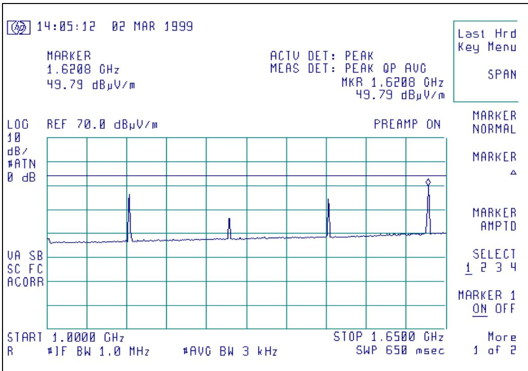
Radiated Emission signature scan, 174 MHz, horizontal polarity, 125 MW level
