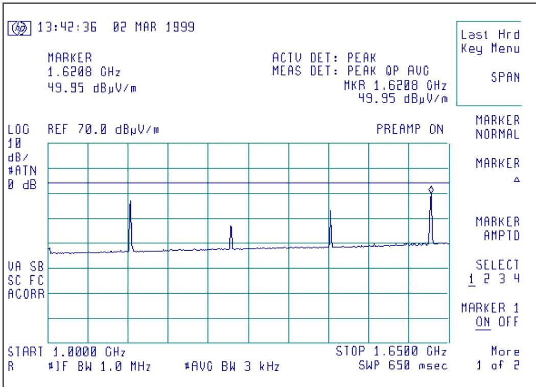
Radiated Emission signature scan, 162 MHz, horizontal polarity, 50 MW level
