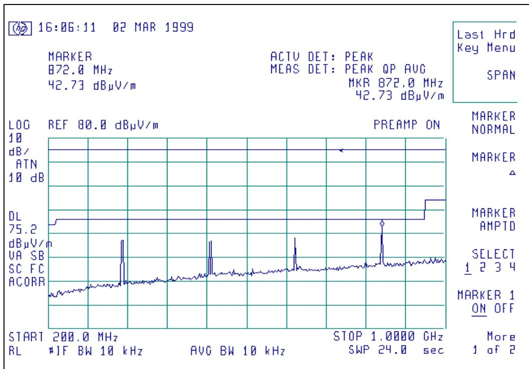
Radiated Emission signature scan, 174 MHz, vertical polarity, 125 MW level
