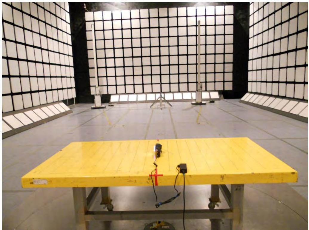
For radiated emissions 30MHz~1GHz
