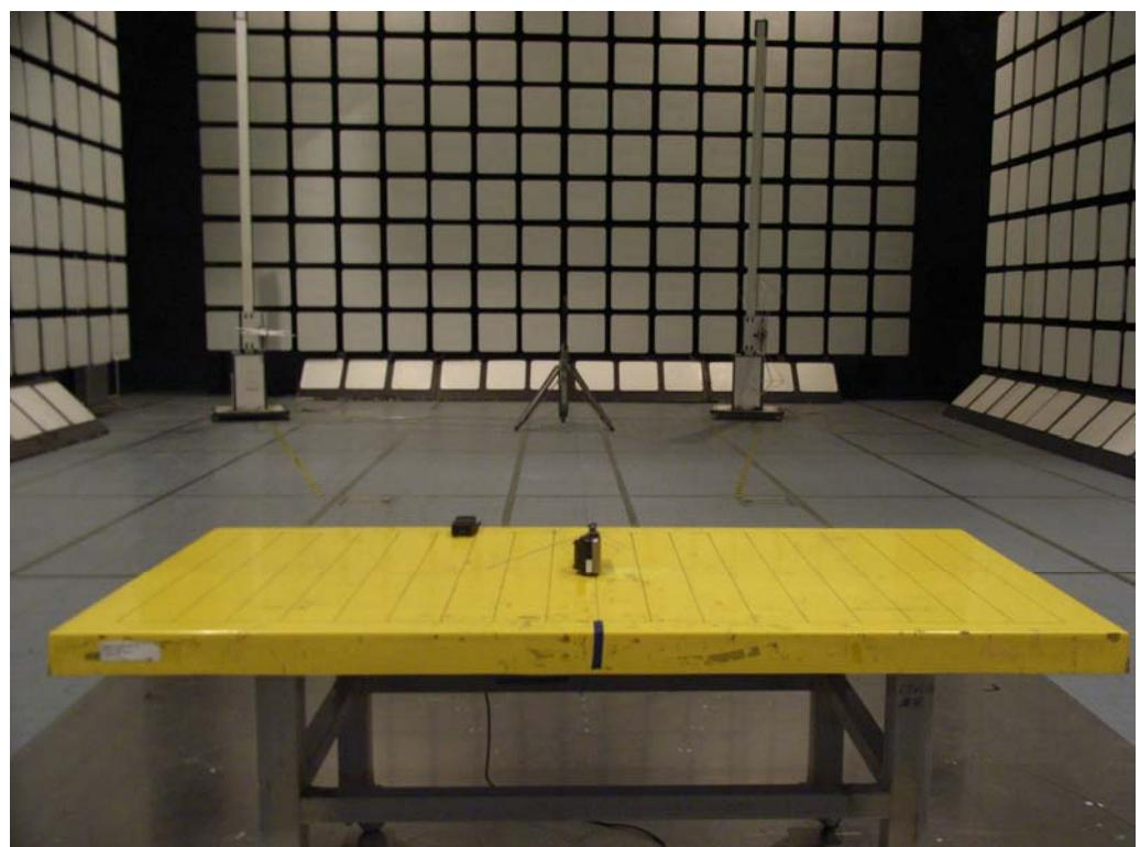
For radiated emissions 30MHz~1GHz
