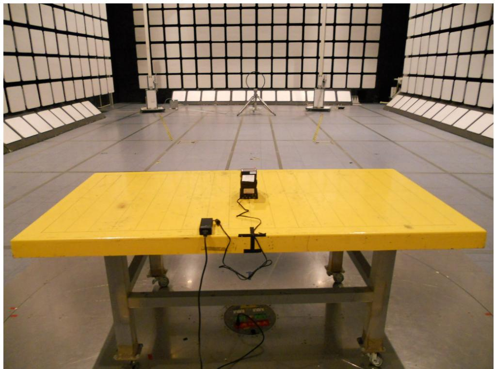
For radiated emissions 30MHz~1GHz
