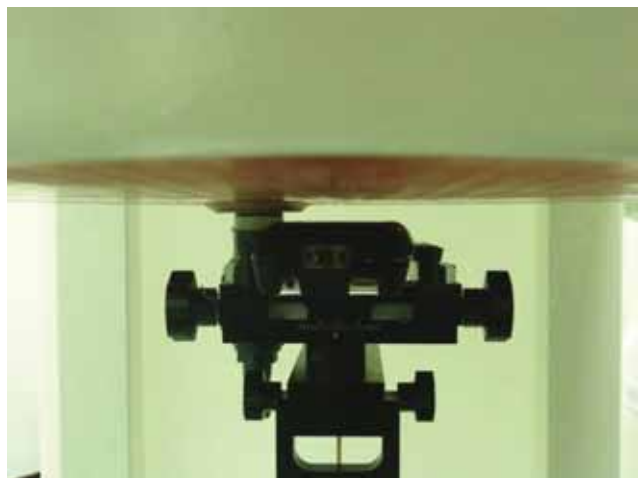
Rear Face of the DUT with Phantom 1 cm Gap
