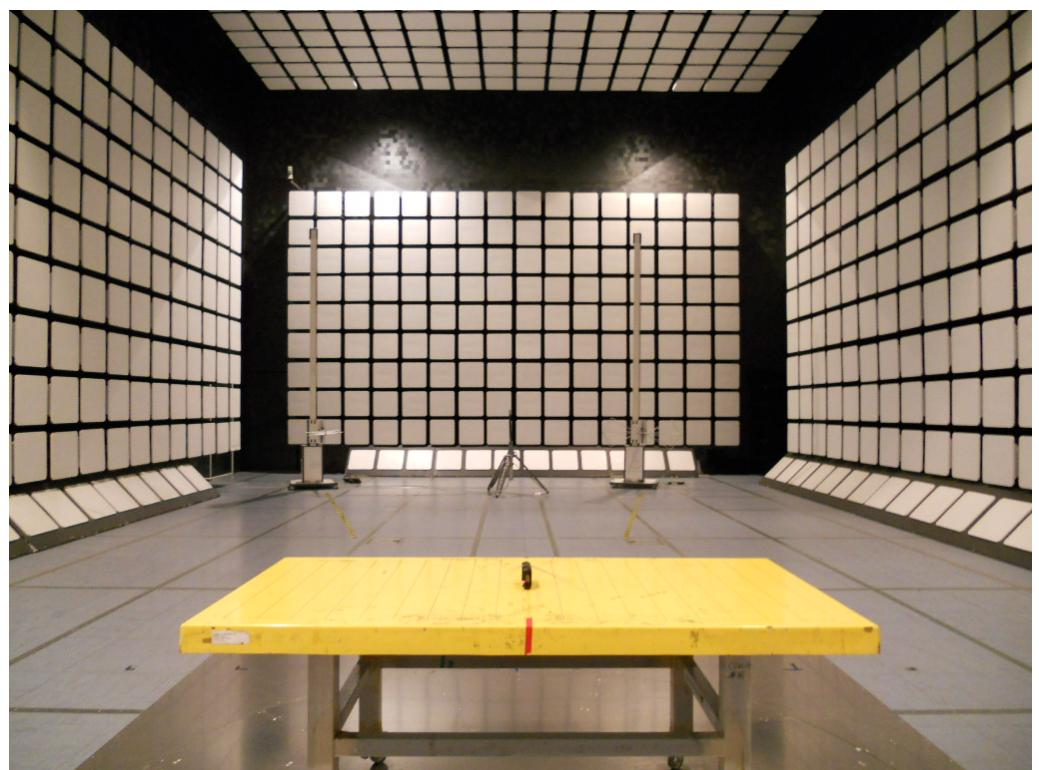
For radiated emissions 30MHz~1GHz
