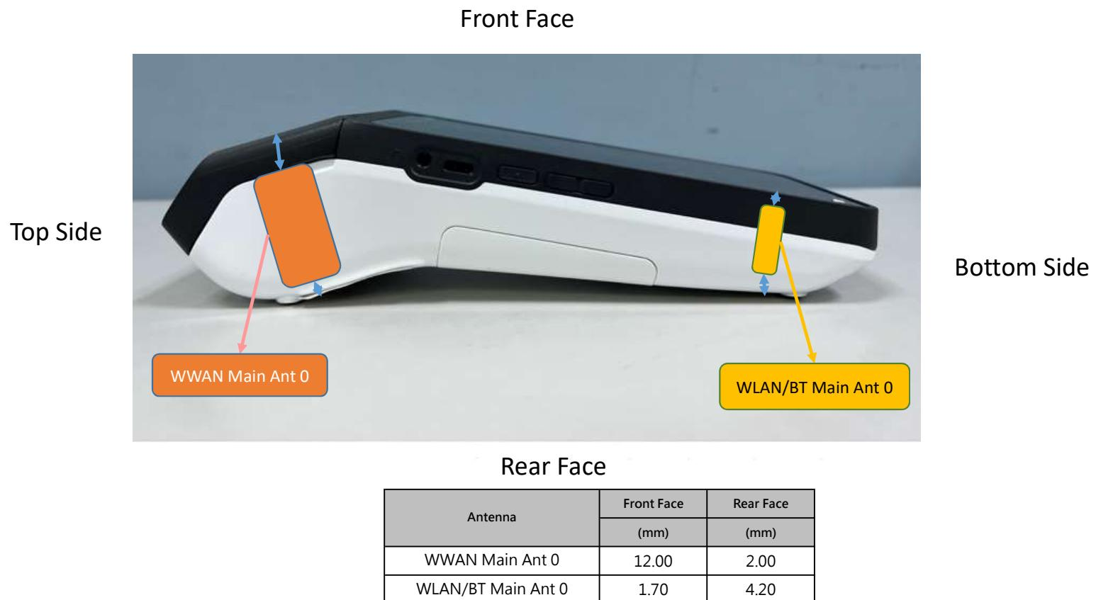
**<Photographs of Extremity SAR Test Setup>**
