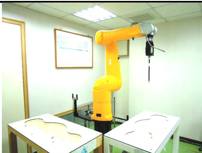
Fig-3.2 SPEAG DASY52 System
