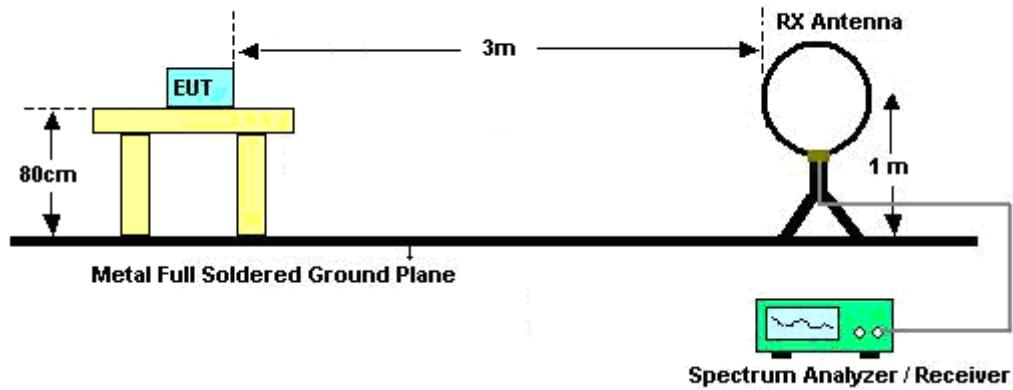
For radiated emissions from 30MHz to 1GHz
