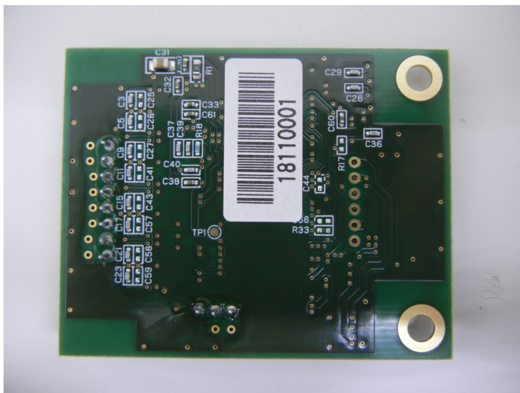
RFID Reader/Writer Board <Rear>
