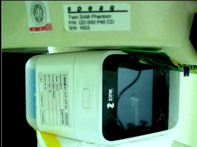
Right Side of EUT with 0 cm Gap
