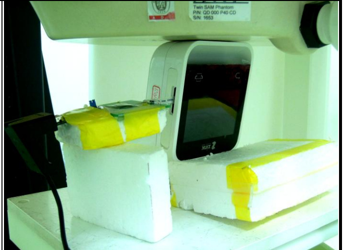
Bottom Side of EUT with 0 cm Gap
