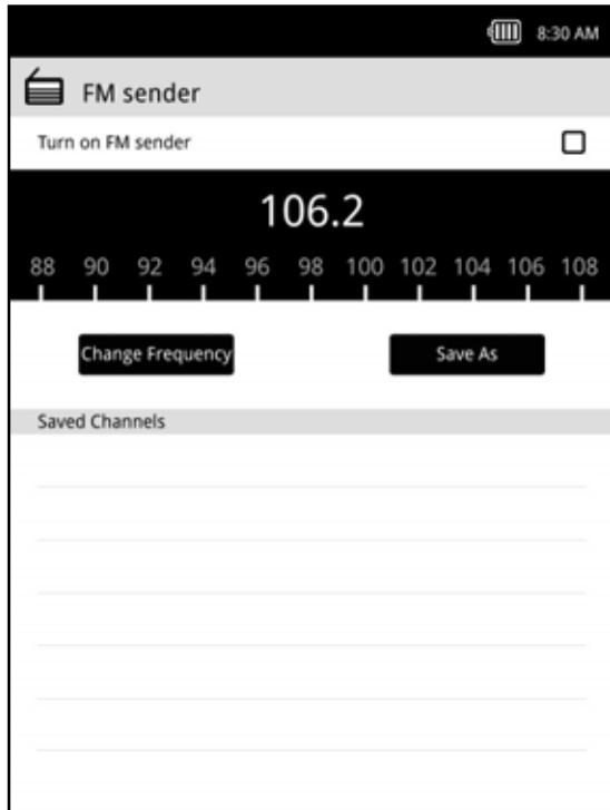
Once the check box has been checked, the FM sender will be activated and will broadcast as the now frequency (like 106.2 in pic)
