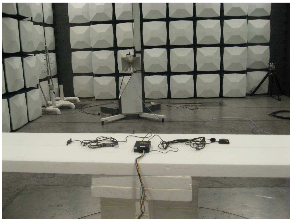
Photograph 4: Set-up for Radiated Emissions (1GHz-18GHz)
