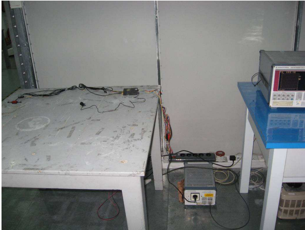
Photograph 2: Set-up for Radiated Emissions, below 30MHz
