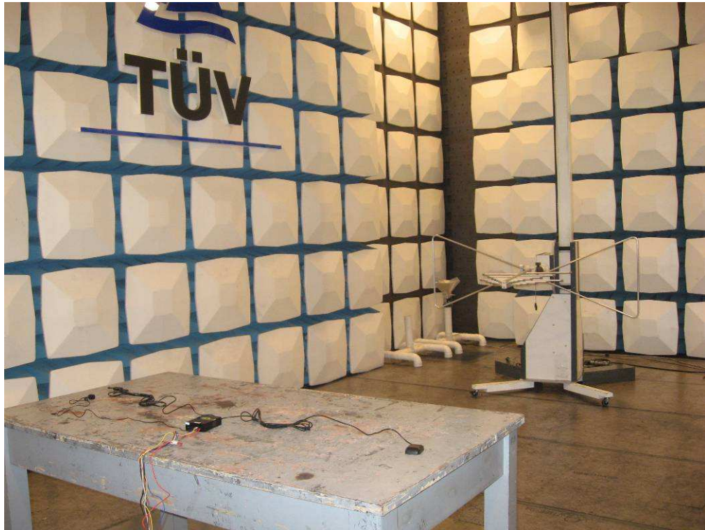
Photograph 4: Set-up for Radiated Emissions (1GHz-18GHz)
