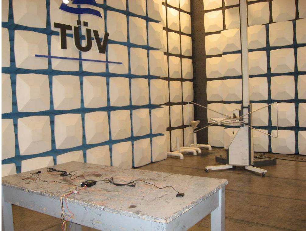
Photograph 2: Set-up for Radiated Emissions, above 1GHz
