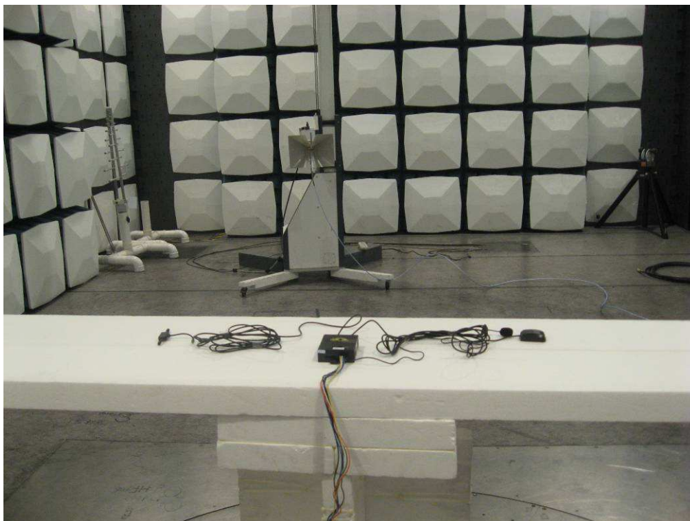
Photograph 6: Set-up for Spurious Emissions (1GHz-18GHz)
