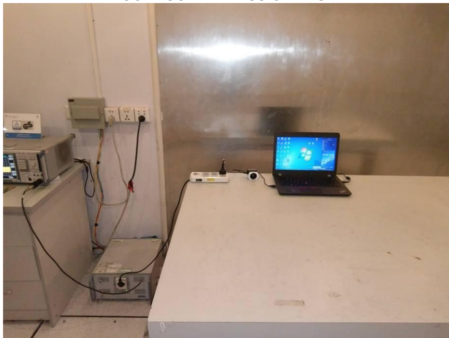
CONDUCTED EMISSION TEST
