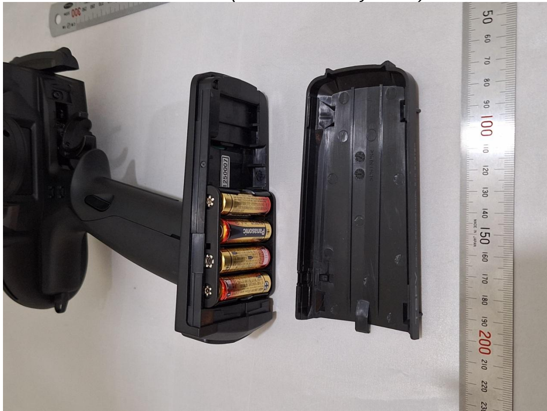
Figure 13 Internal View (Removed Battery Cover) with AAA Battery Type
