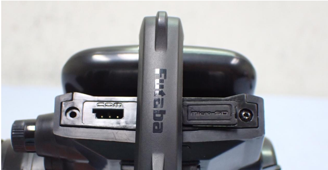
Figure 10 Internal View -Communication port & microSD port
