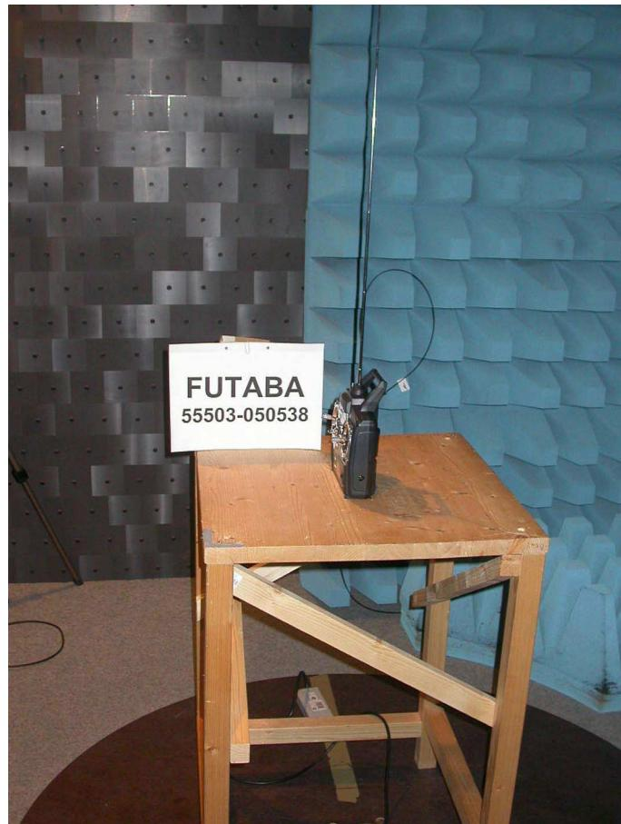
**Test setup for radiated emission measurement
