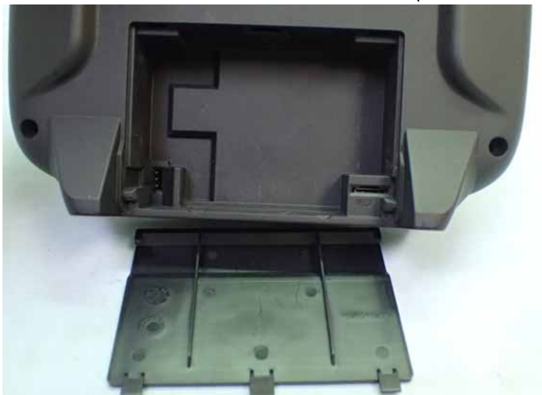
Figure 7 Internal View (Removed Battery Cover)
