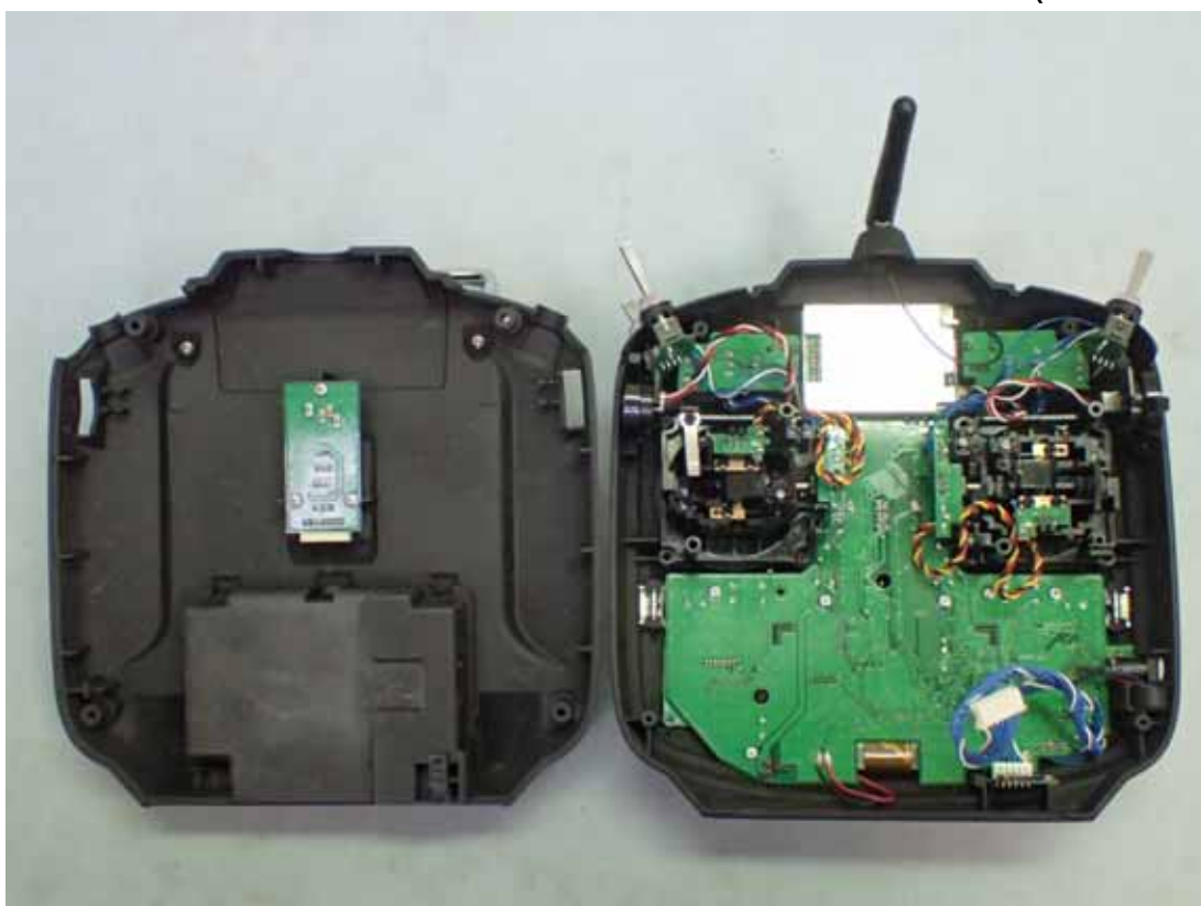
Figure 8 Internal View (Removed Covers)
