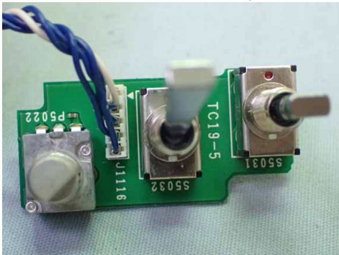
Figure 21 Internal View (Control Board, Front View)
