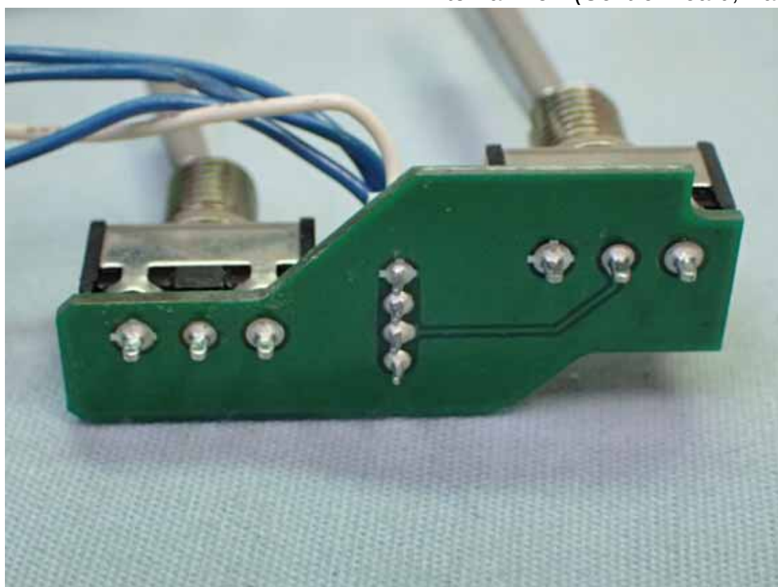
Figure 20 Internal View (Control Board, Back View)
