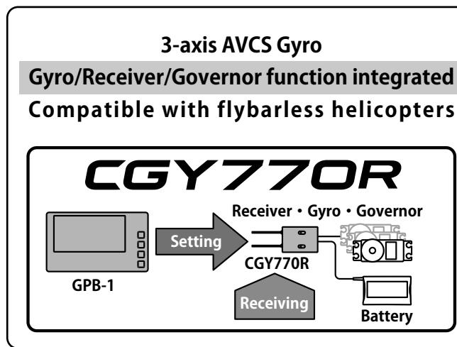
Futaba CGY770R is gyro, 3-axis Stabilization System combining AVCS gyro and head speed governor and receiver in one box designed for flybarless helicopters. Its cutting edge MEMS (Micro Electro Mechanical System) sensor design, ultra high-speed processing speed, and advanced PID control algorithm put it a league of its own ahead of all ahead of all other heading hold gyros in size, weight and performance.
