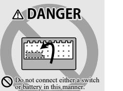
∅ Do not connect either a switch or battery in this manner.
