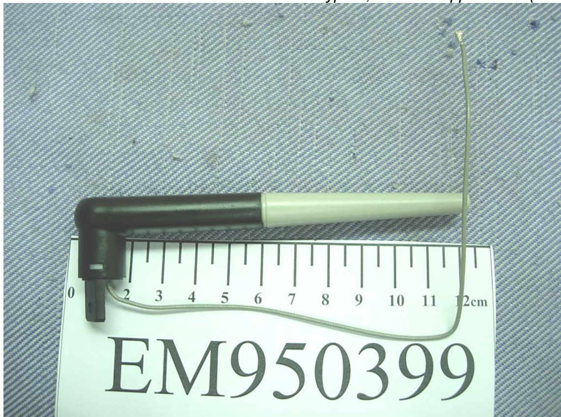
Figure 14 Antenna Type B, General Appearance (Side View)
