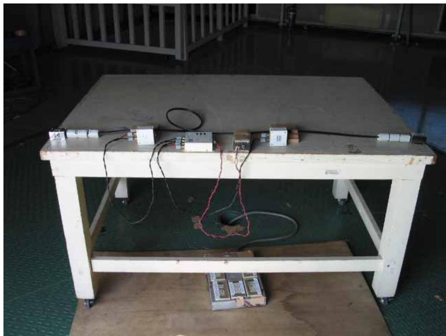
**8.2b** Setup with the Maximized RFI Field Strength Emission Level
