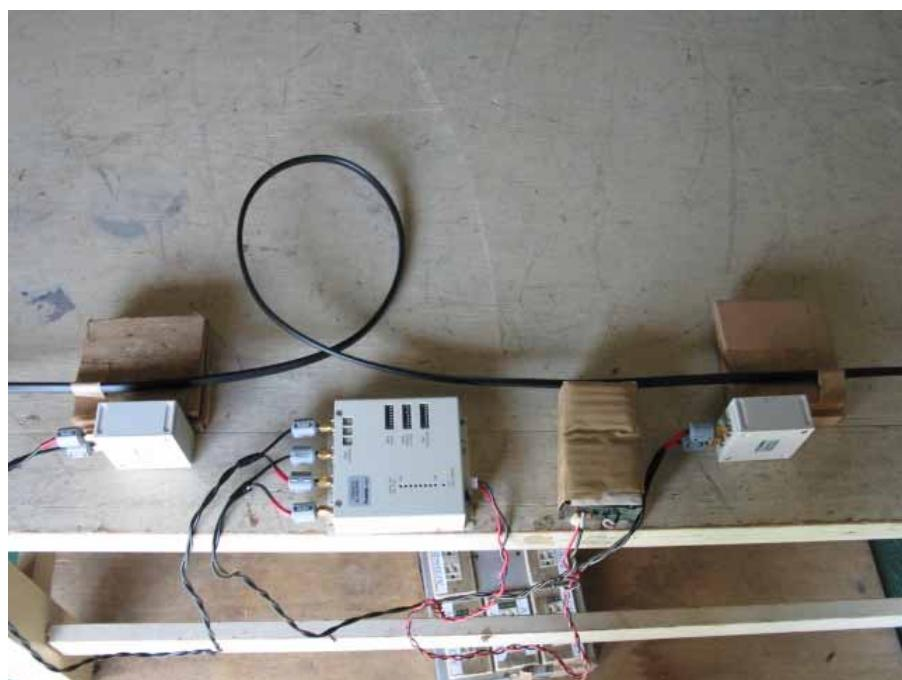
**8.3a** Setup with the Maximized RFI Field Strength Emission Level
