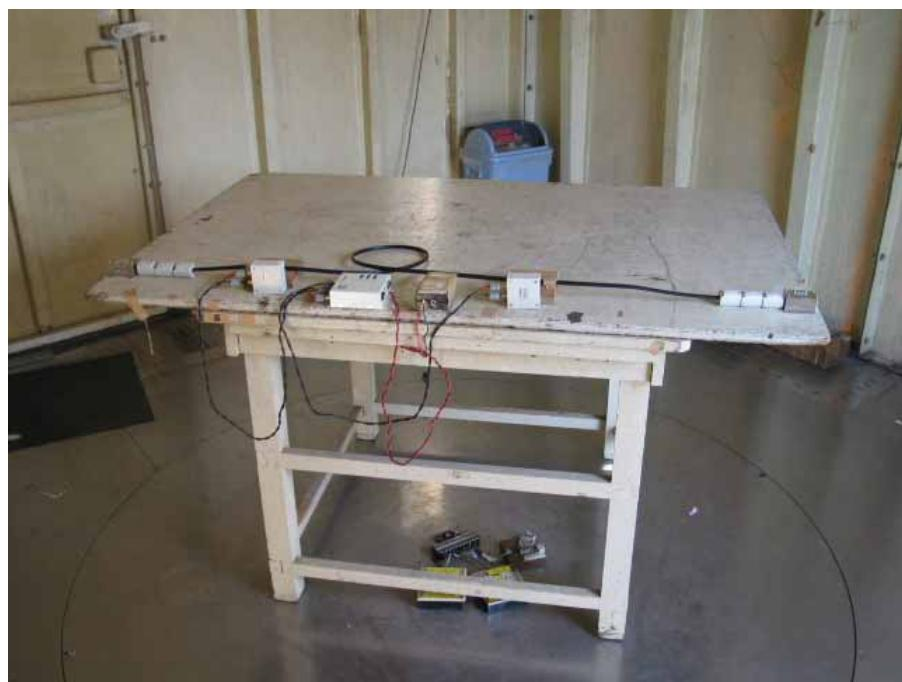
**8.3b** Setup with the Maximized RFI Field Strength Emission Level
