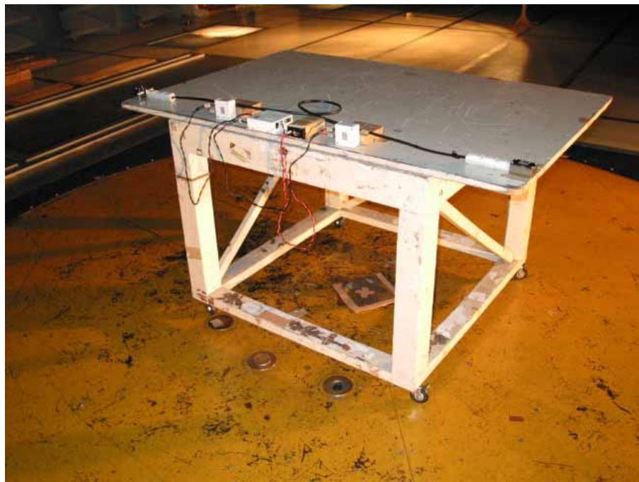
**8.1b** Setup with the Maximized RFI Field Strength Emission Level
