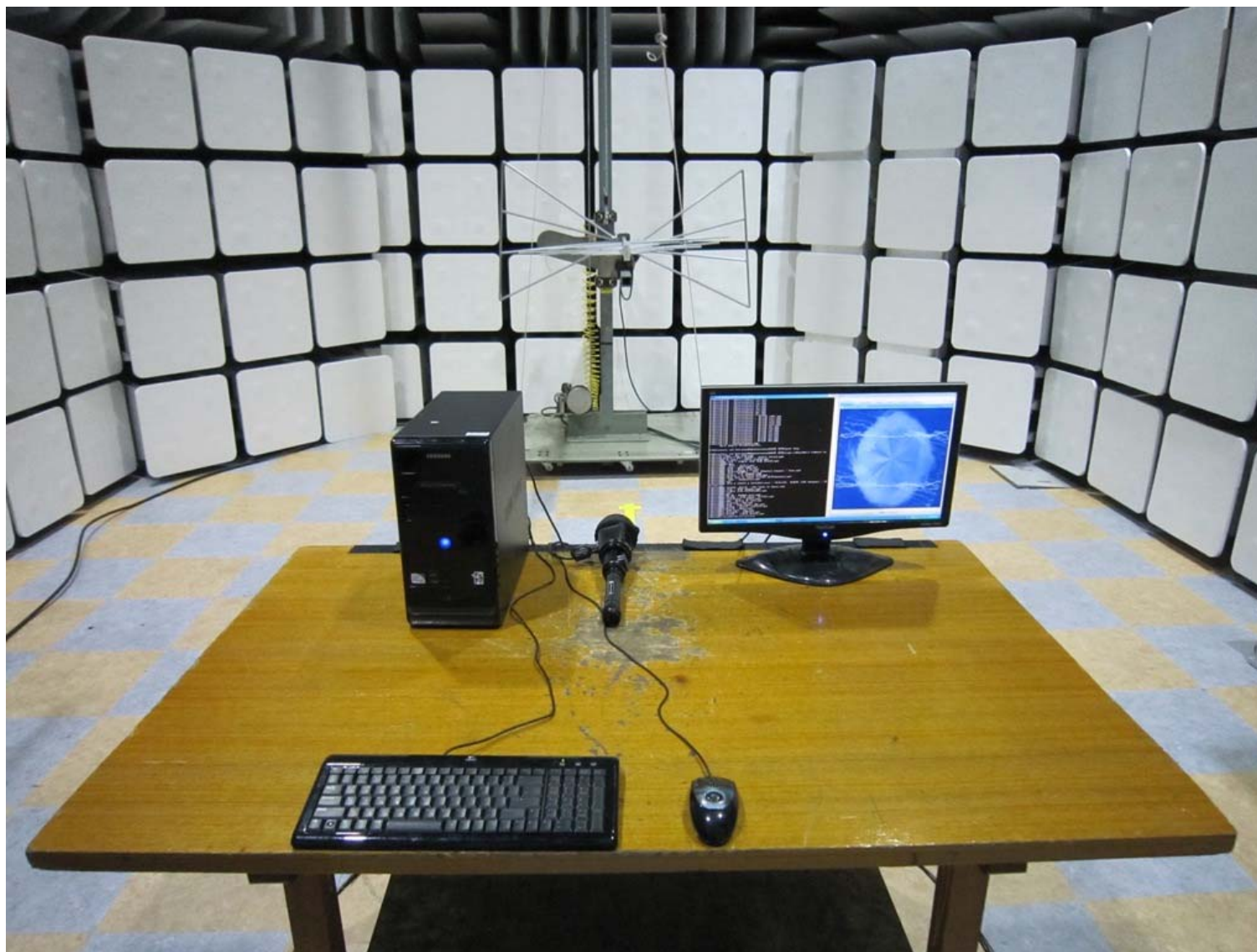
Radiated_30 MHz to 1 GHz_USB Data Up/Down & LED Lighting Mode_Front View
