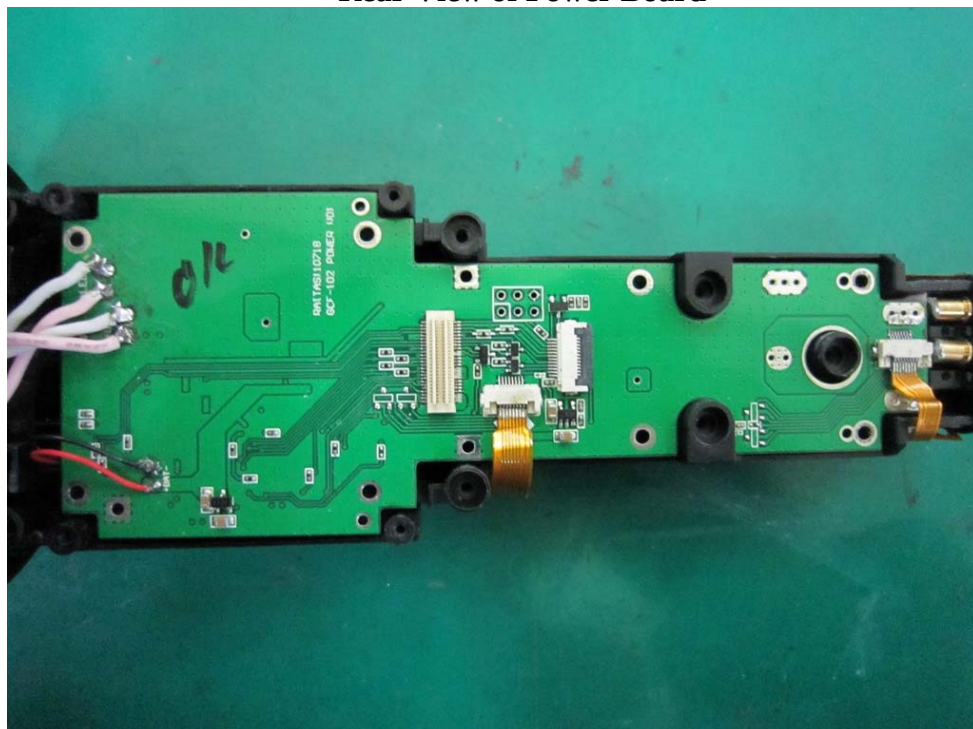
Rear View of Power Board
