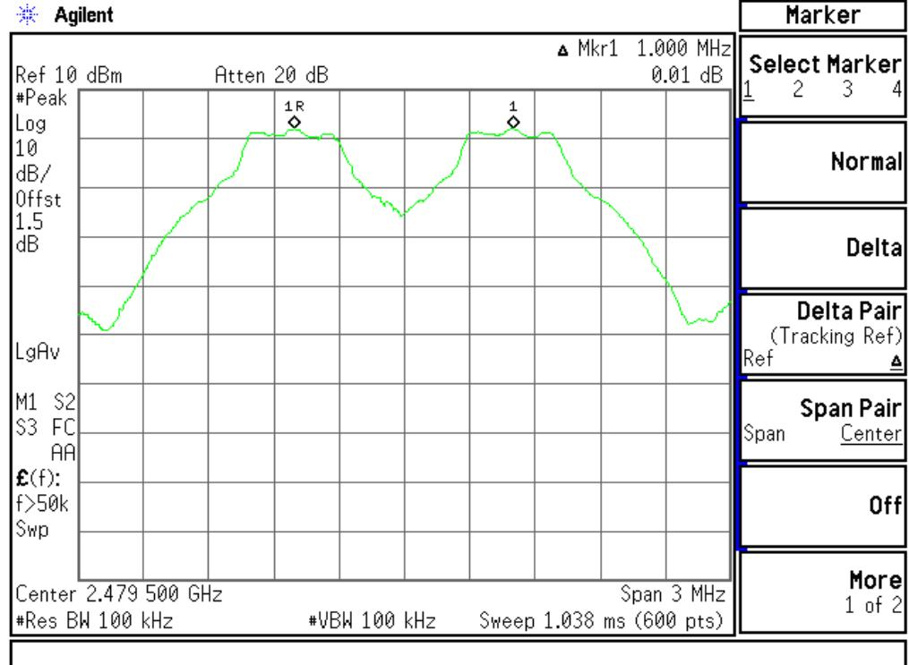
**Measurement of 20dB Bandwidth****Test frequency: 2402MHz**
