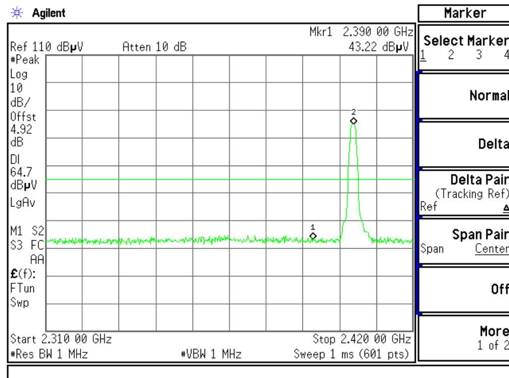
**Band Edges (CH High)****Detector mode: Peak****Polarity: Vertical**
