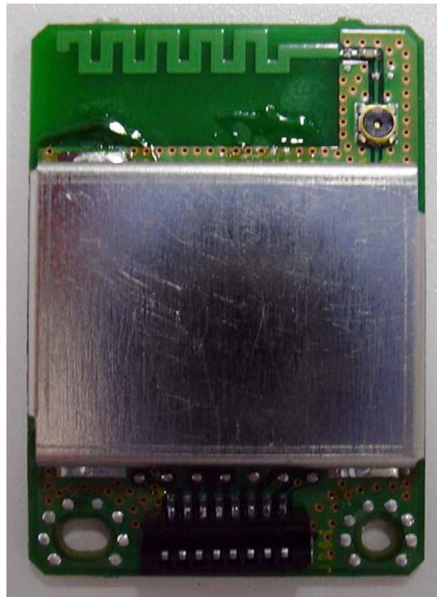
The UFL connector is used for testing only.
