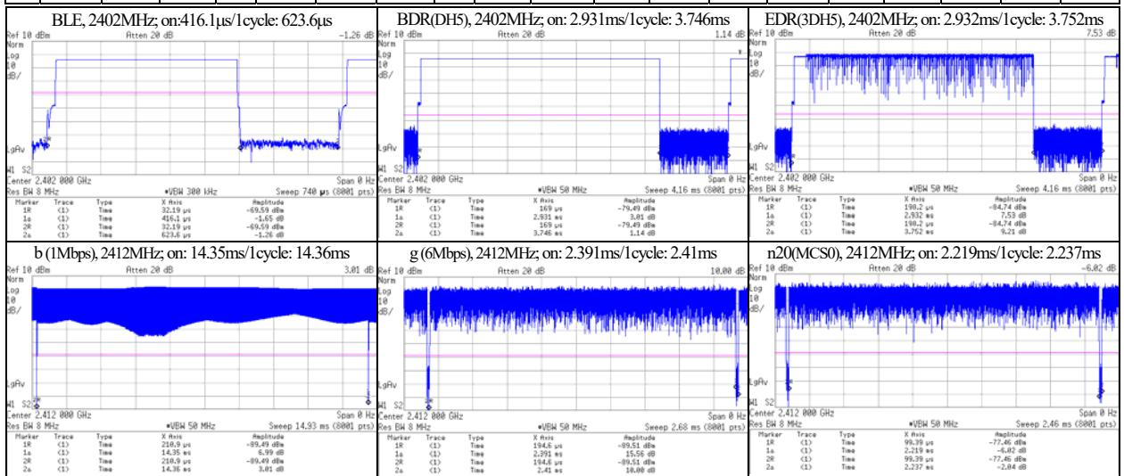
\*. Calculating formula: Result-Time average power (dBm) = (P/M Reading, dBm)+(Cable loss, dB)+(Attenuator, dB)
