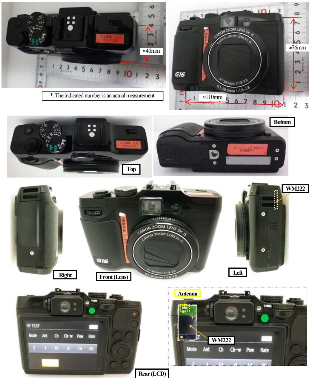
Photograph of Wireless module and antenna
