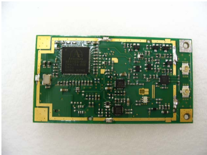
WLAN module Top Shield off
