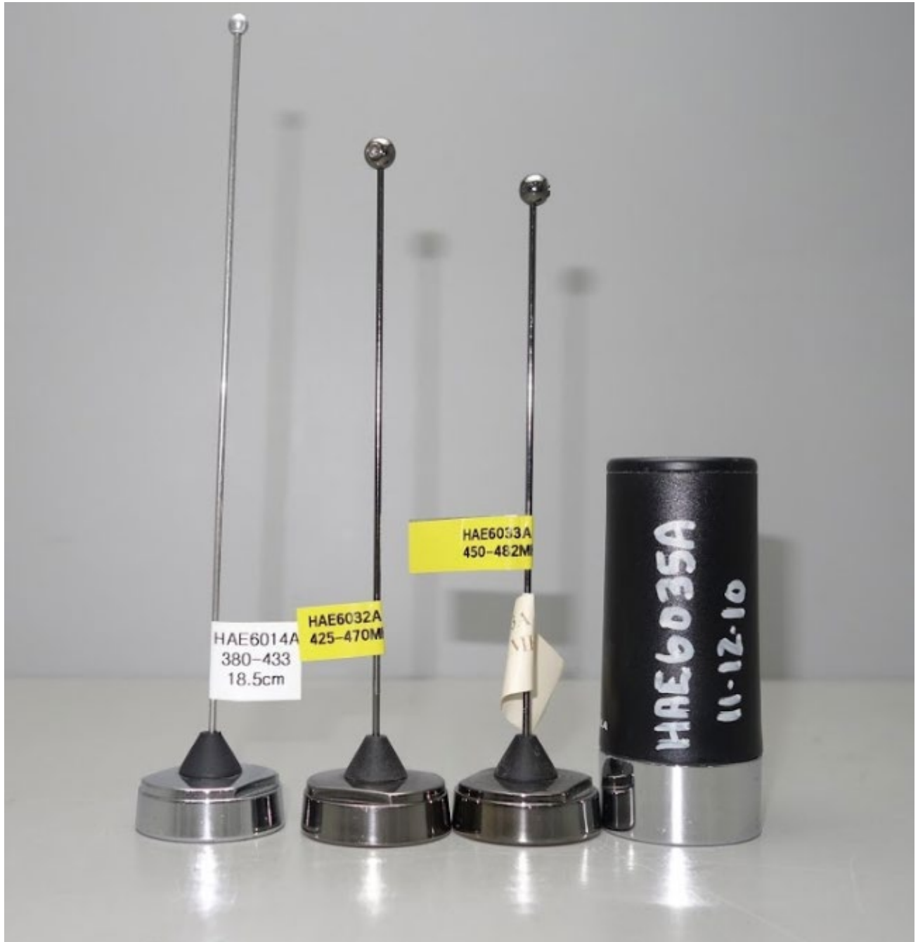
Antenna kit numbers, from left to right; HAE4014A, HAE6032A, HAE6033A, and HAE6035A
