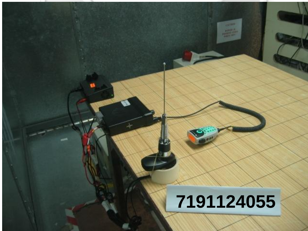
Conducted Emissions Test Setup (Rear View)
