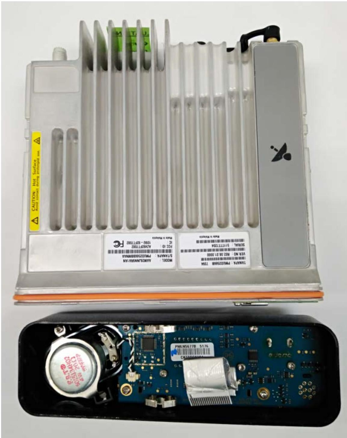
Chassis and control head (Bottom)
