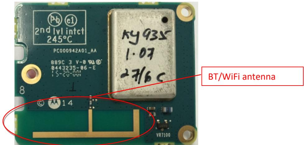
Wifi/GPS/BT board with Shield (Bottom)
