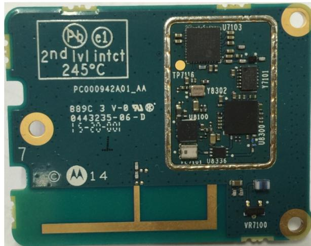
Wifi/GPS/BT board without Shield (Bottom)
