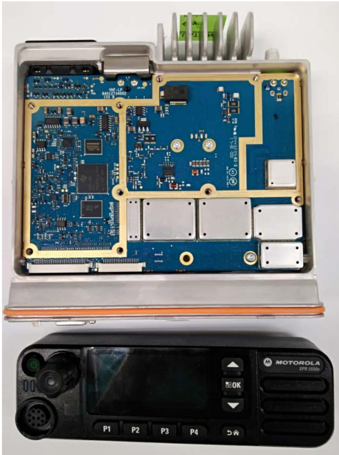
RF boards with chassis and control head (Top)
