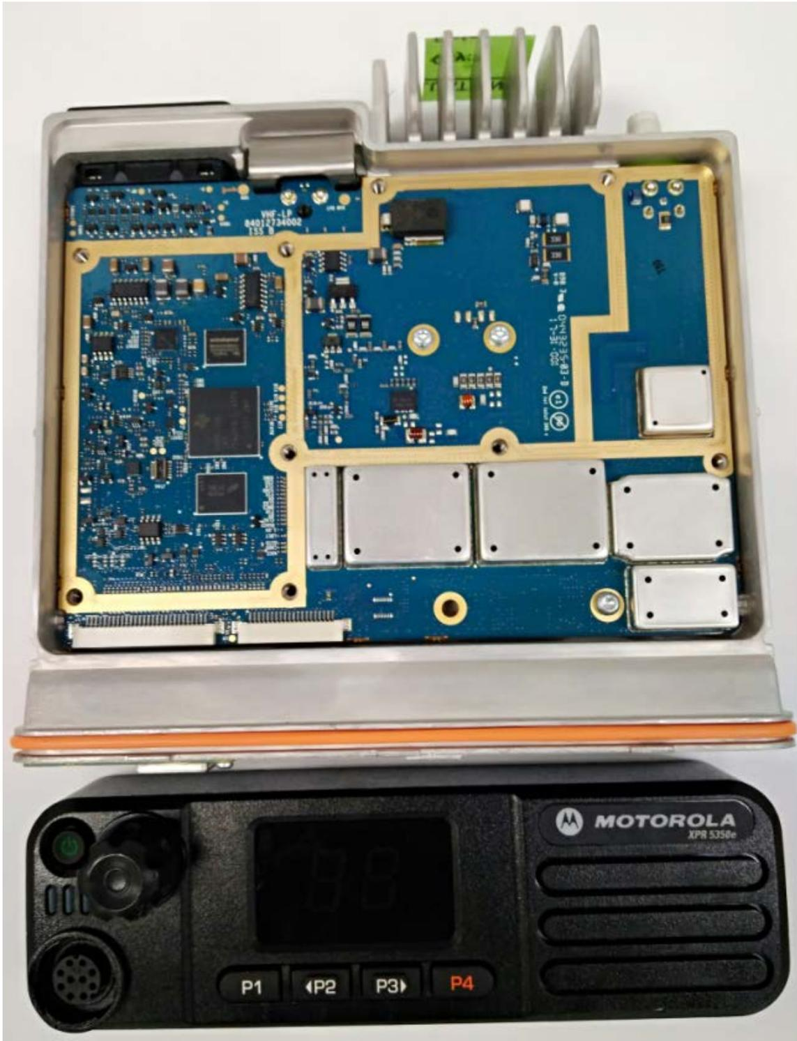
RF boards with chassis and control head (Top)
