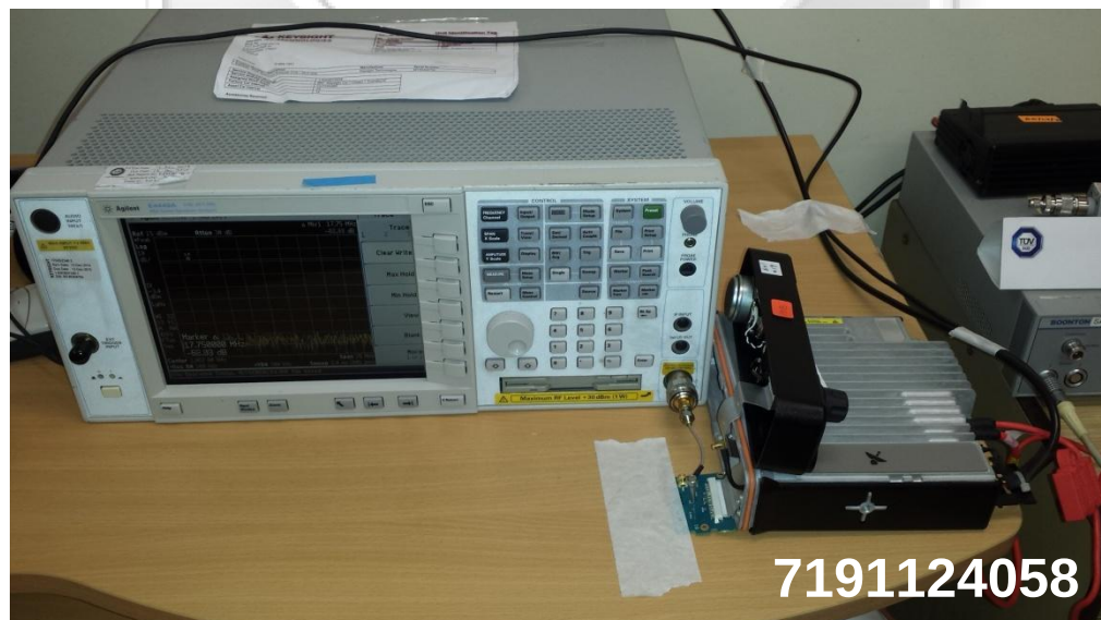
Average Frequency Dwell Time Test Setup
