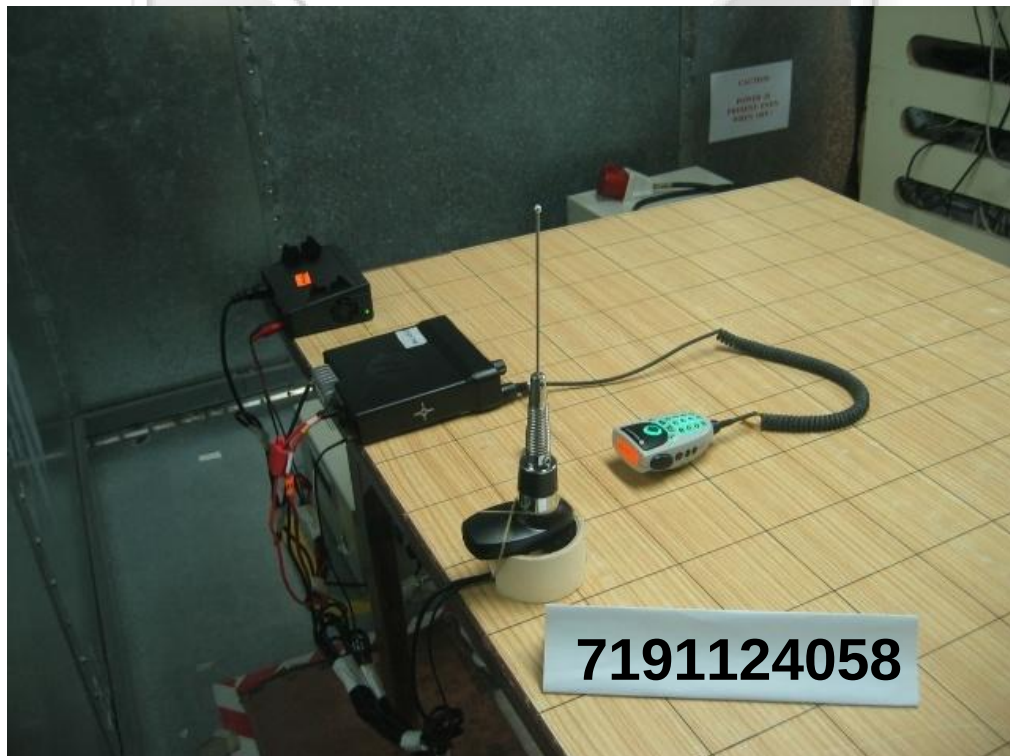
Conducted Emissions Test Setup (Rear View)
