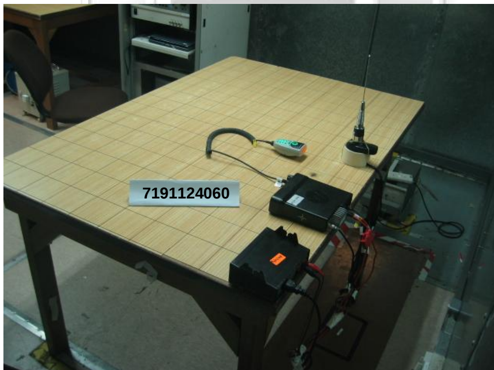
Conducted Emissions Test Setup (Rear View)
