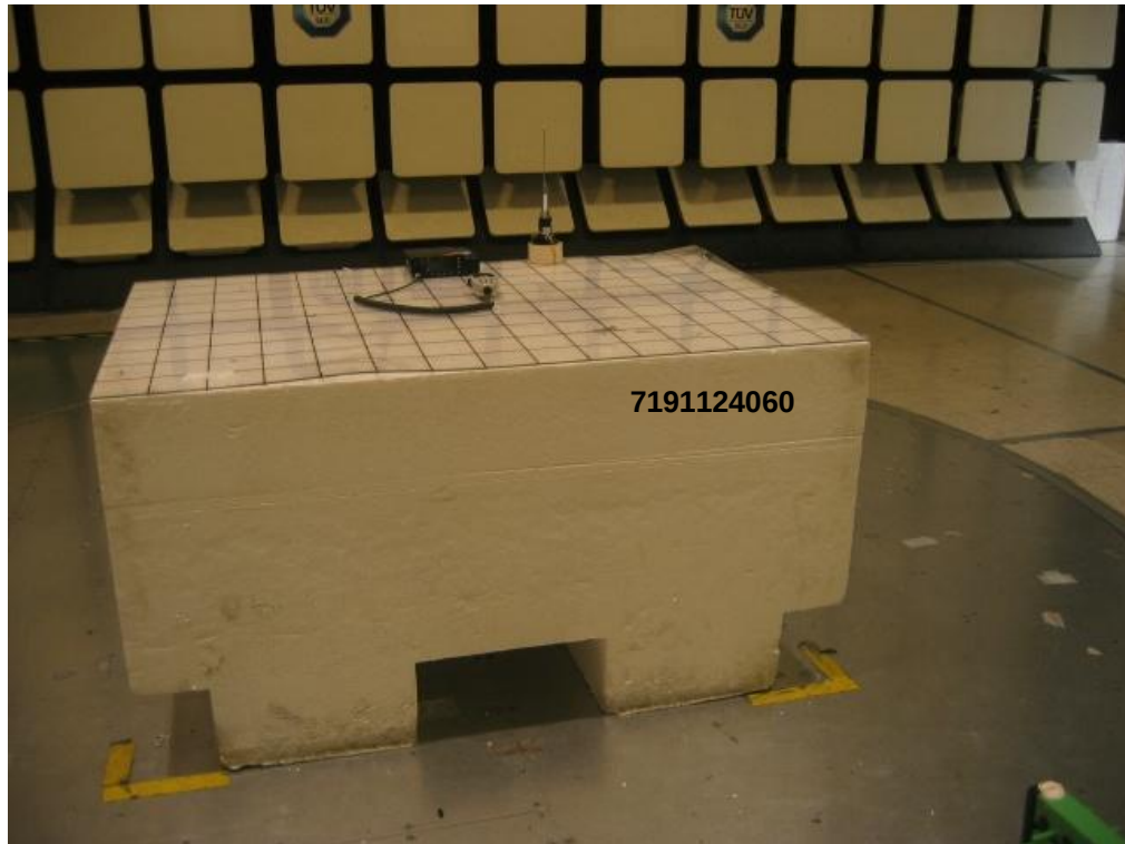
Radiated Emissions Test Setup (Front View)
