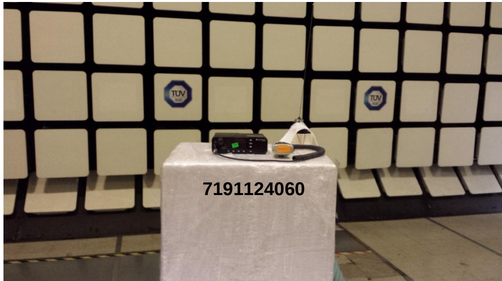
Radiated Emissions Test Setup (Front View)
