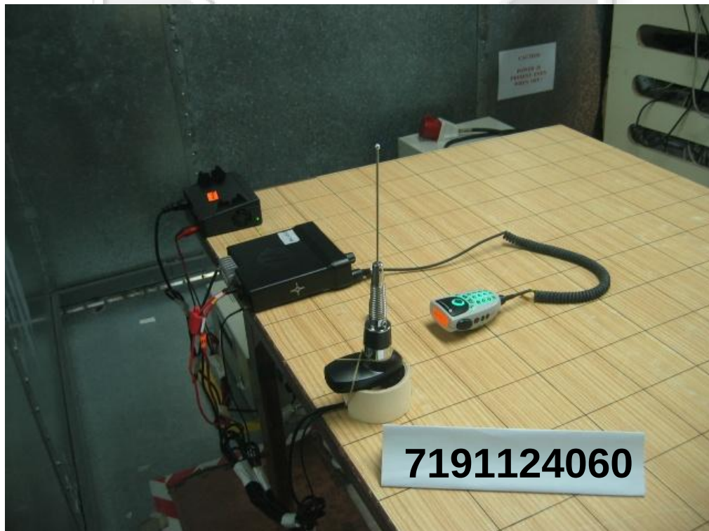
Conducted Emissions Test Setup (Rear View)
