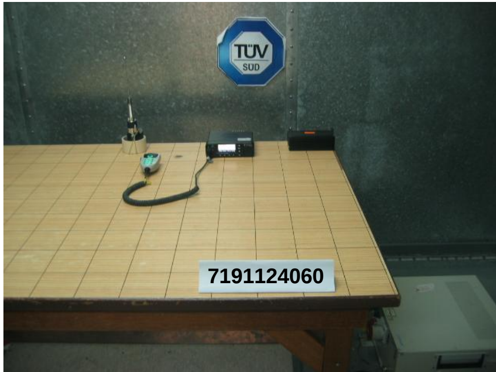
Conducted Emissions Test Setup (Front View)
