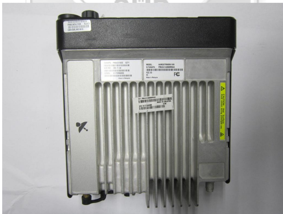
Physical Location of FCC, IC Label on EUT
