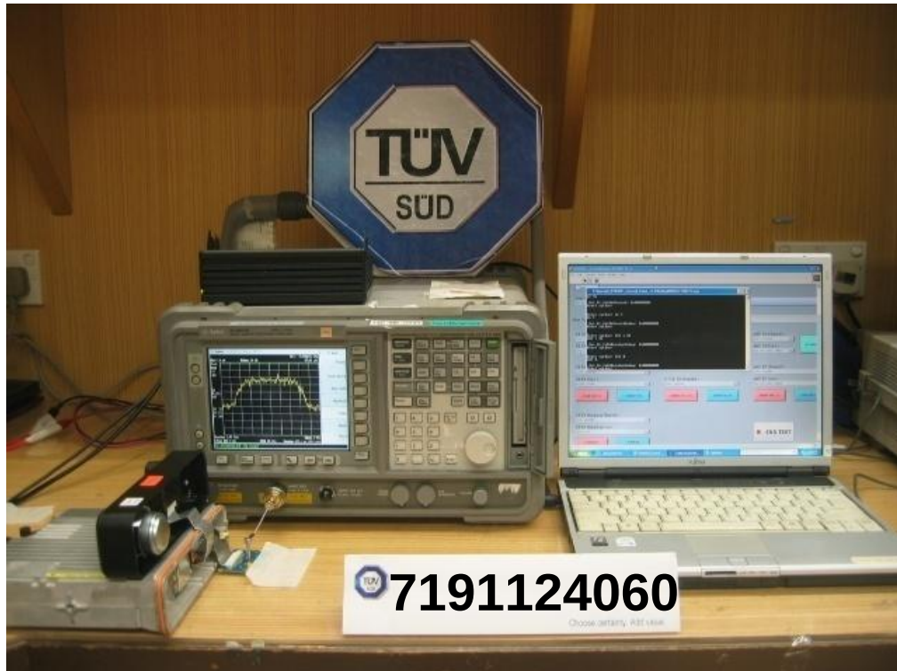
Band Edge Compliance (Conducted) Test Setup
