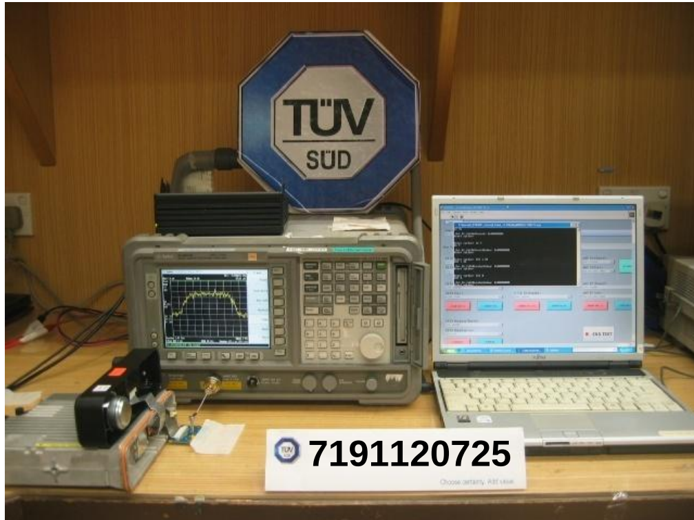
Carrier Frequency Separation Test Setup
