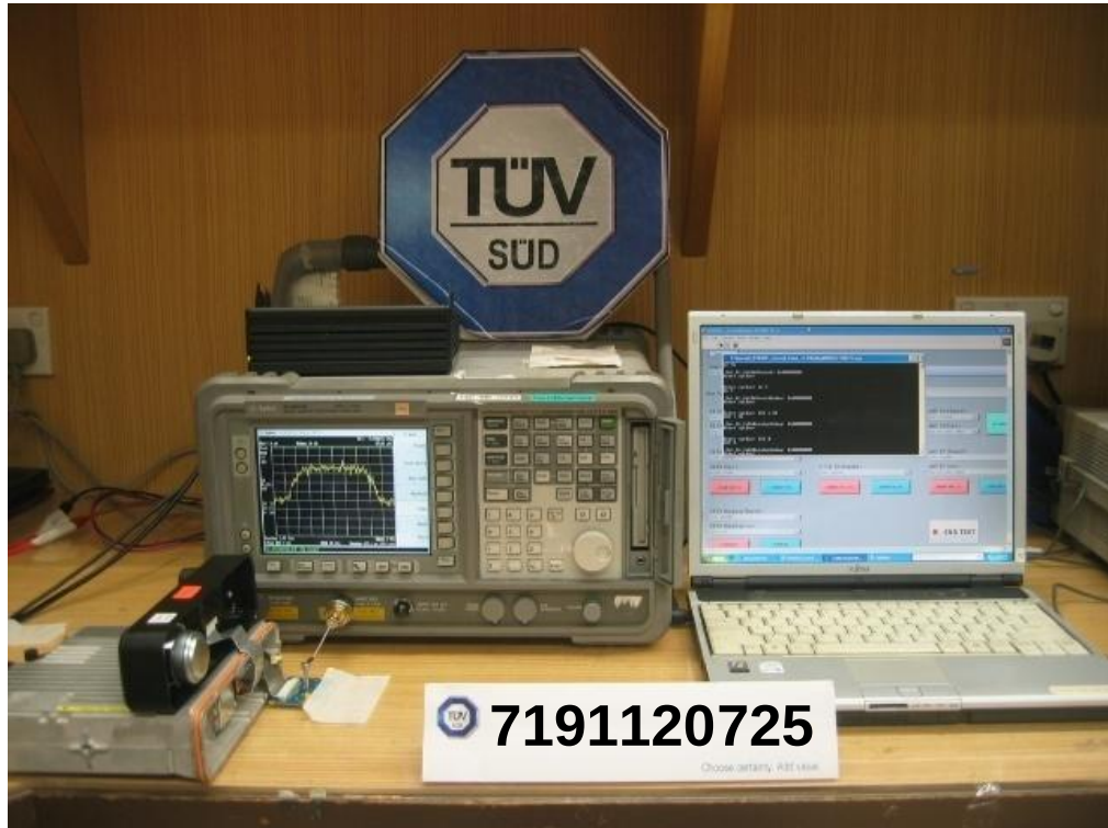
Band Edge Compliance (Conducted) Test Setup
