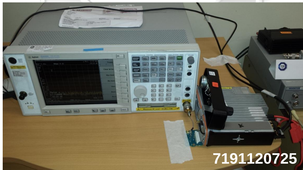
Average Frequency Dwell Time Test Setup
