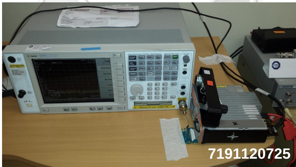
RF Conducted Spurious Emissions Test Setup
