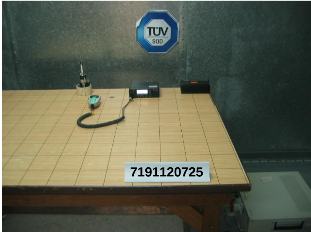
Conducted Emissions Test Setup (Front View)
