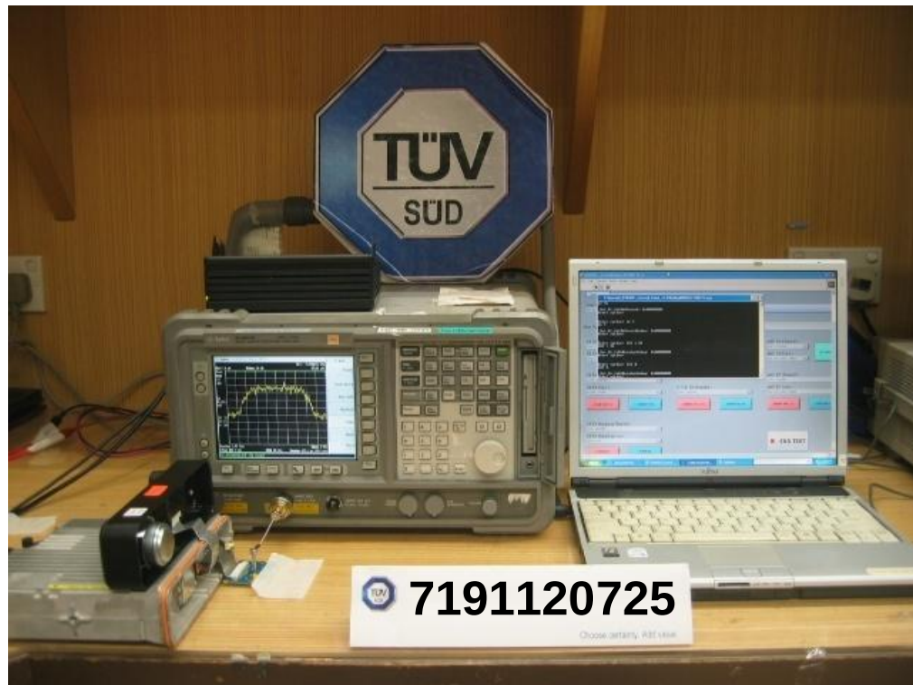
Peak Power Spectral Density Test Setup
