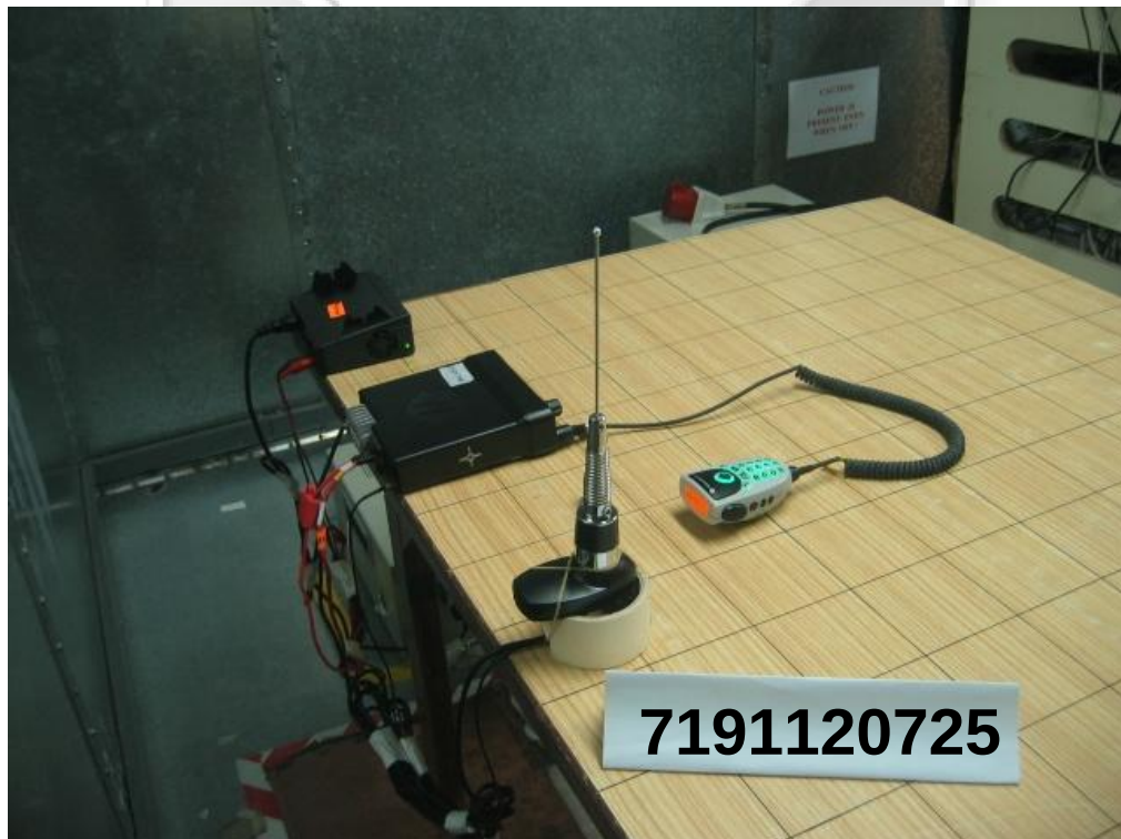
Conducted Emissions Test Setup (Rear View)
