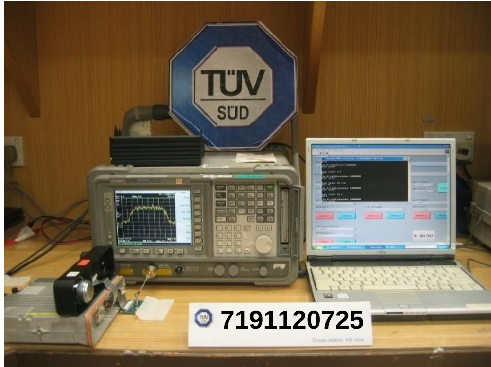
Number of Hopping Frequencies Test Setup
