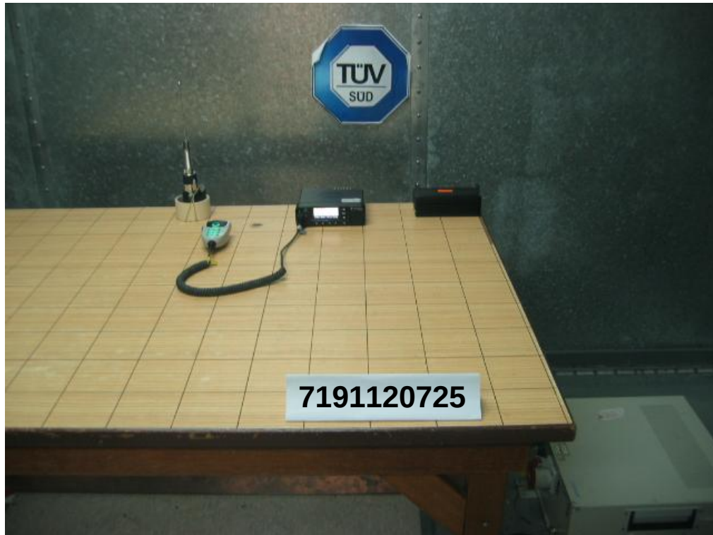
Conducted Emissions Test Setup (Front View)
