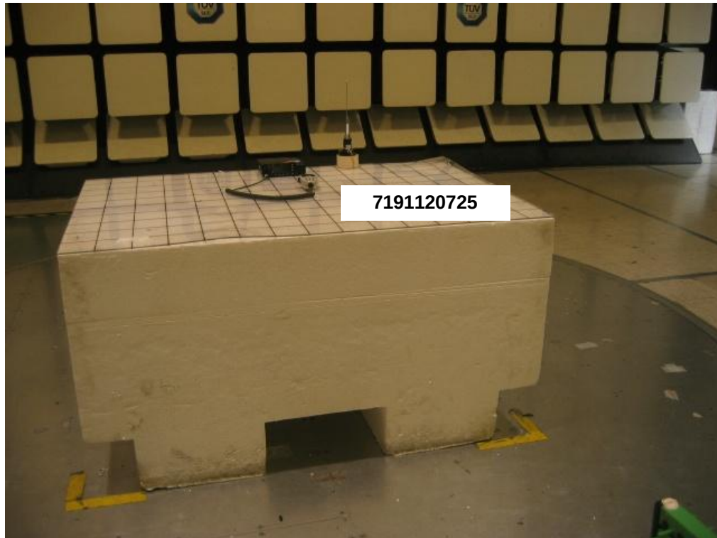
Radiated Emissions Test Setup (Front View)
