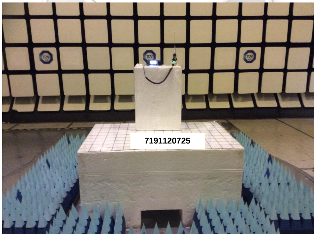
Band Edge Compliance (Radiated) Test Setup
