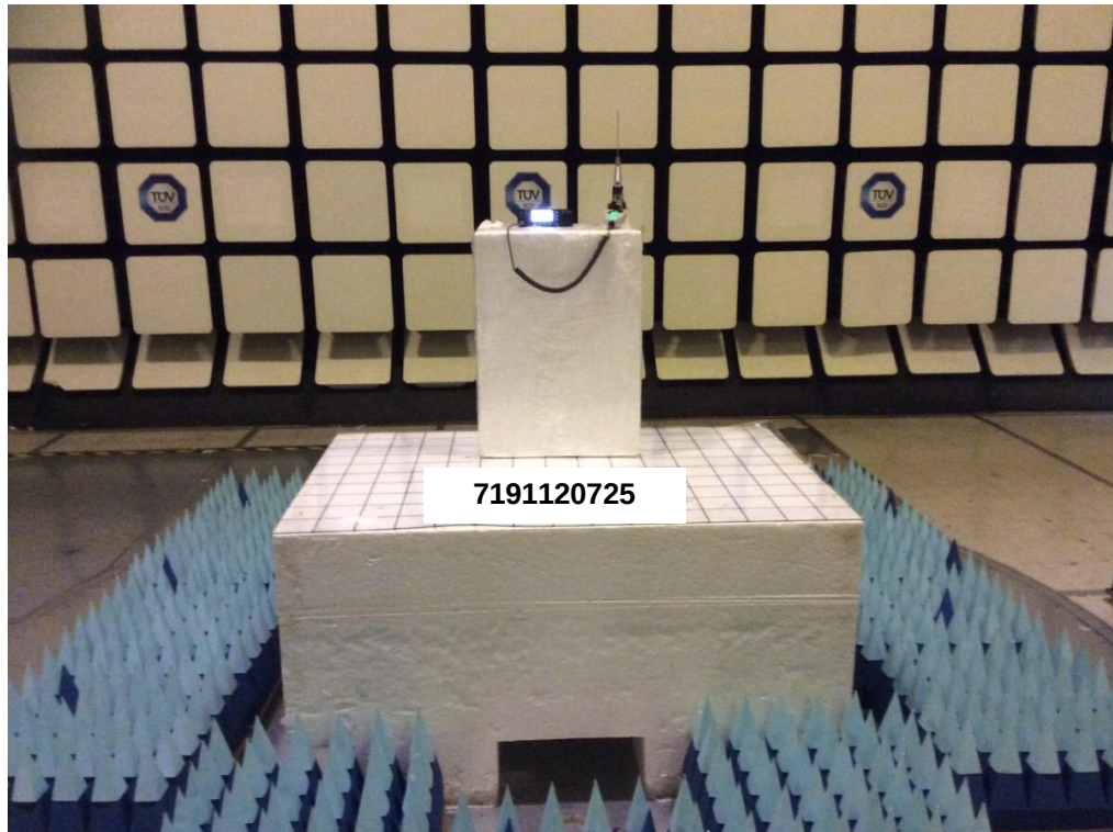
Radiated Emissions Test Setup (Front View)
