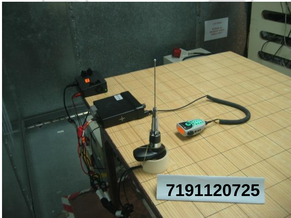
Conducted Emissions Test Setup (Rear View)
