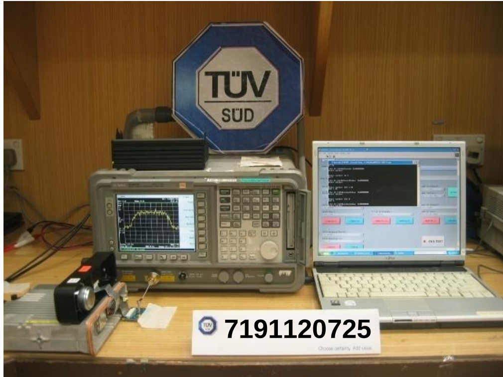
Spectrum Bandwidth (6dB Bandwidth Measurement) Test Setup
