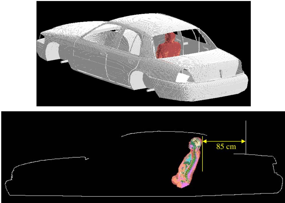
**Figure 2: Passenger model exposed to a trunk-mount antenna: XFDTD geometry.**
