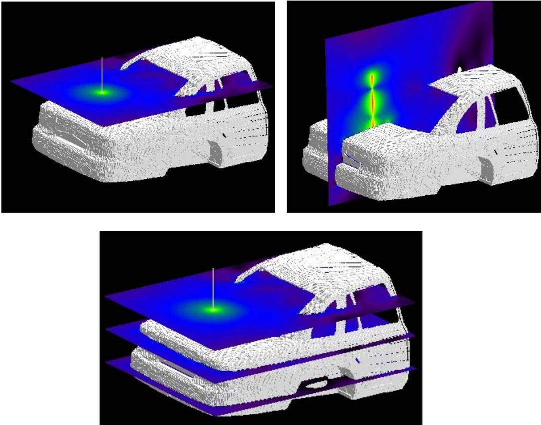
The equivalent power density (S) is computed from the E-field. The following table reports the E-field values computed by XFDTD™ at the three locations, and the corresponding power density.
