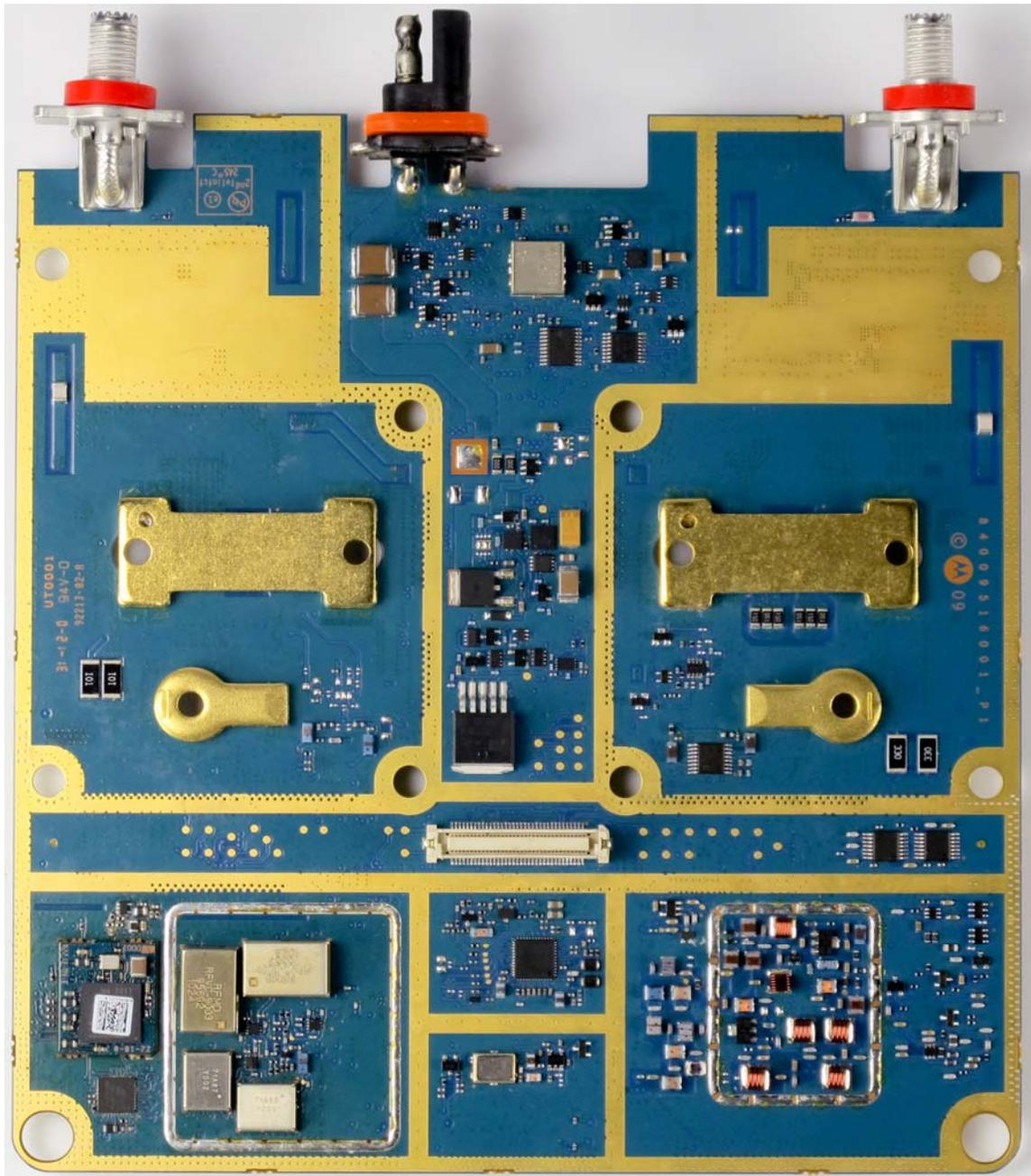
RF BOARD, LESS SHIELD (BOTTOM VIEW)
