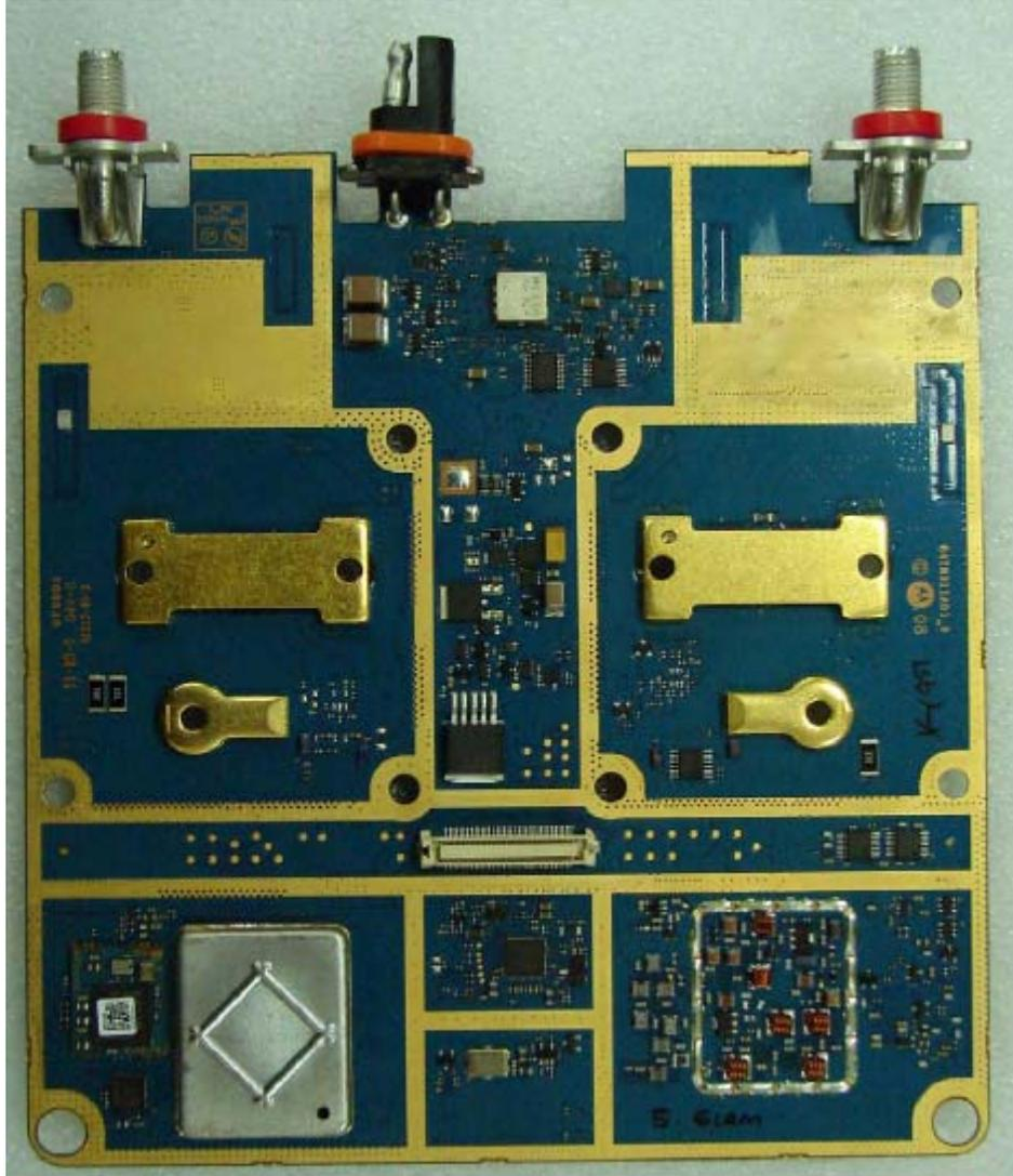
RF board without Shields (Bottom)
