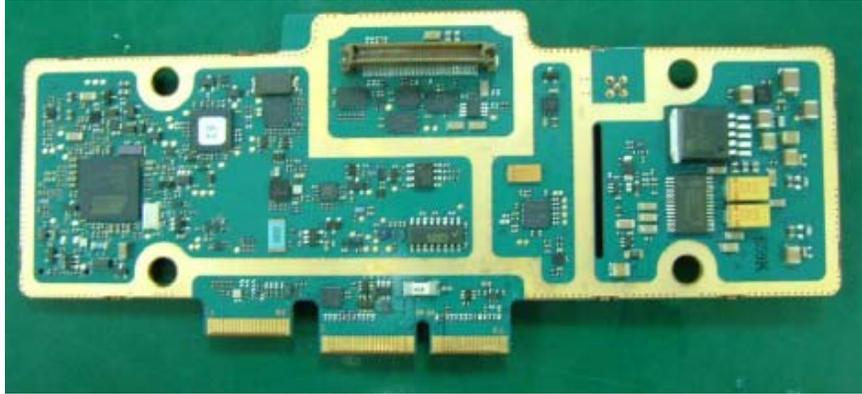
Controller board with Shields (Top)
