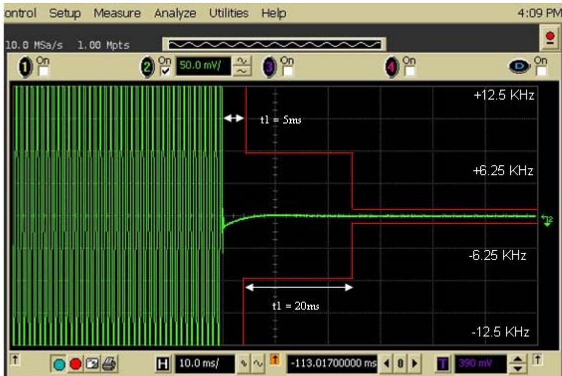
Figure 6K-3: Transient Frequency Behavior, 155.0125MHz, 12.5 KHz Channel Spacing, Key Up Transient
