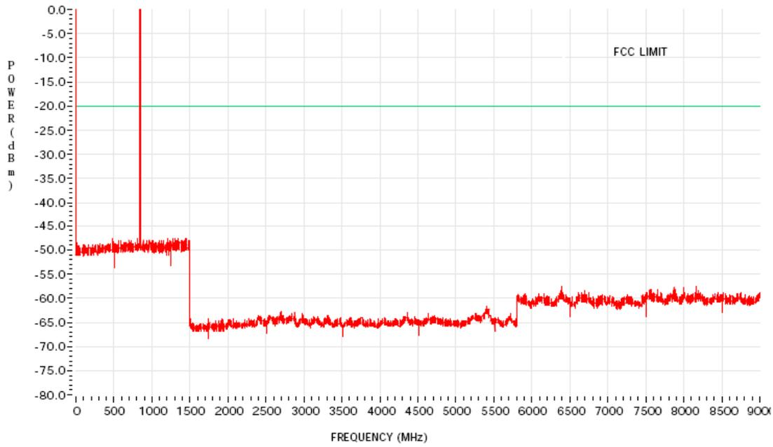
Figure 6G-29: 43 Watts Harmonic of Carrier 868.8875MHz
