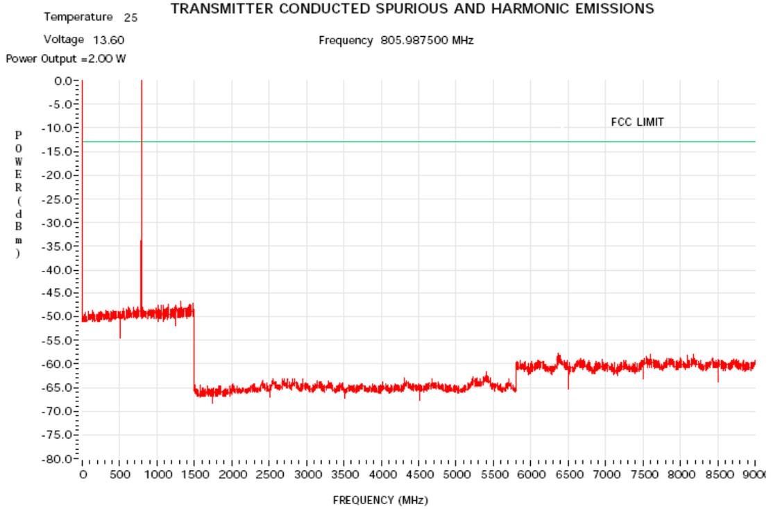
Figure 6G-17: 2 Watts Harmonic of Carrier 805.9875 MHz
