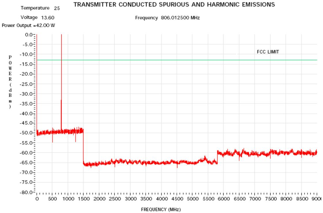
Figure 6G-18: 42 Watts Harmonic of Carrier 806.0125 MHz
