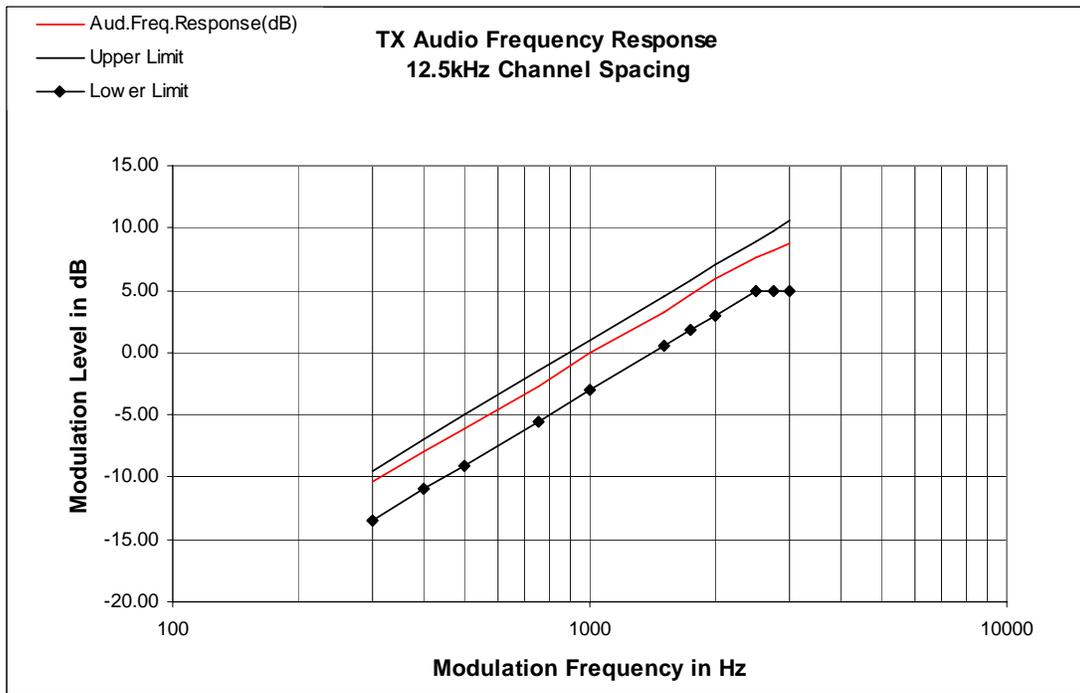
Figure 6B-1: 12.5 KHz Channel Spacing, 155.0125 MHz, Transmit Audio Frequency Response
