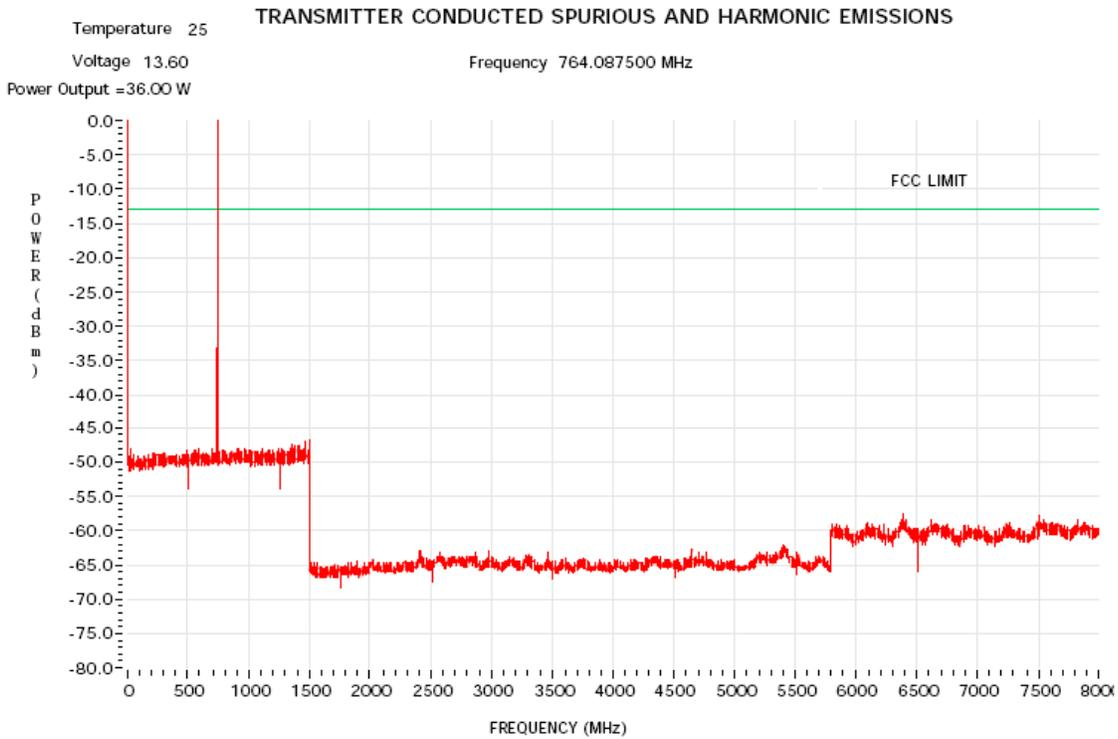
Figure 6G-14: 36 Watts Harmonic of Carrier 764.0875 MHz
