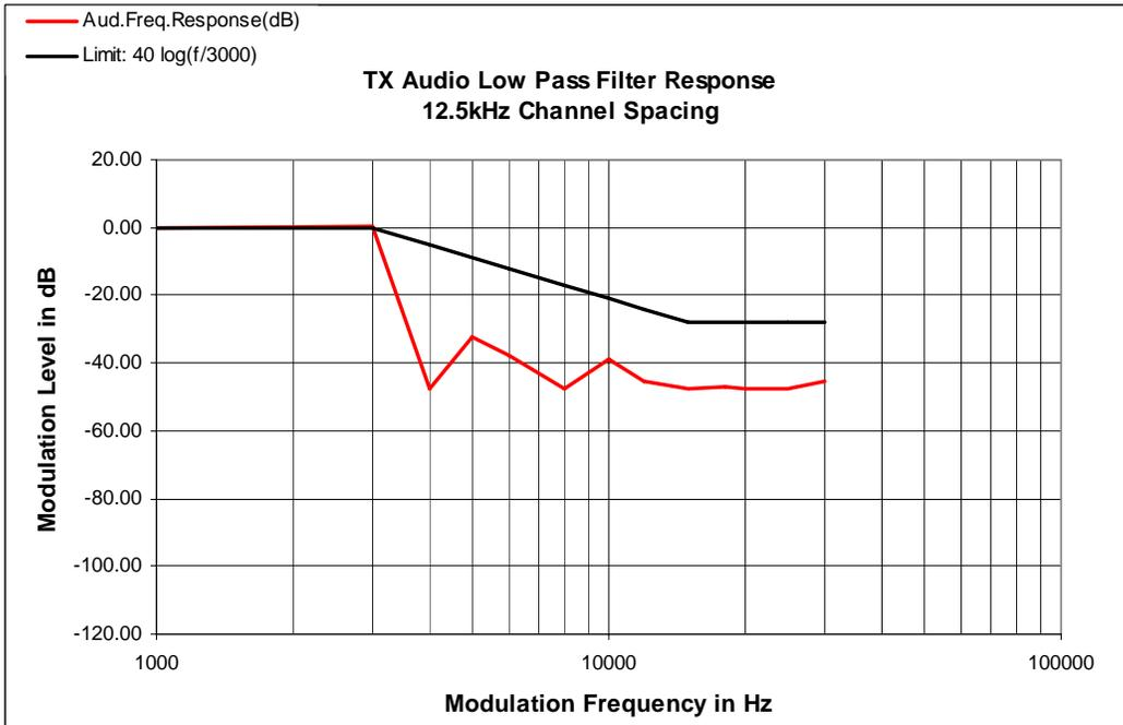
**Figure 6C-1:** 12.5 KHz Channel Spacing, 155.025 MHz, Transmit Audio Low Pass Filter Response
