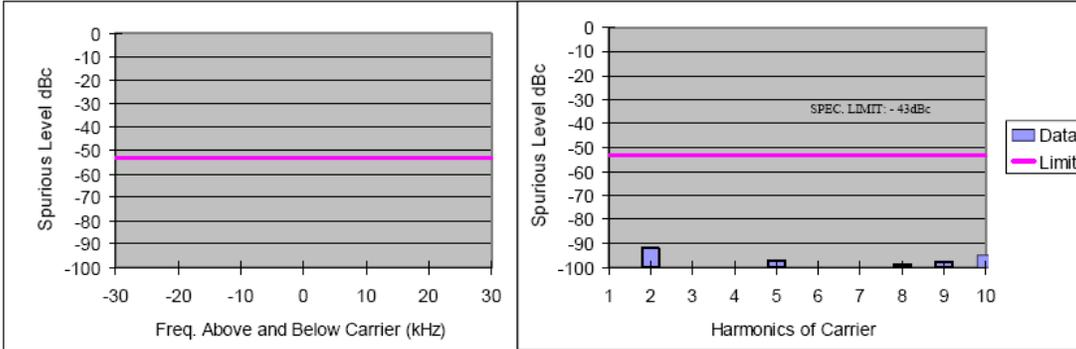
Figure 6G-8: 11 Watt Harmonic of Carrier 155.025 MHz, 25 KHz Channel Spacing
