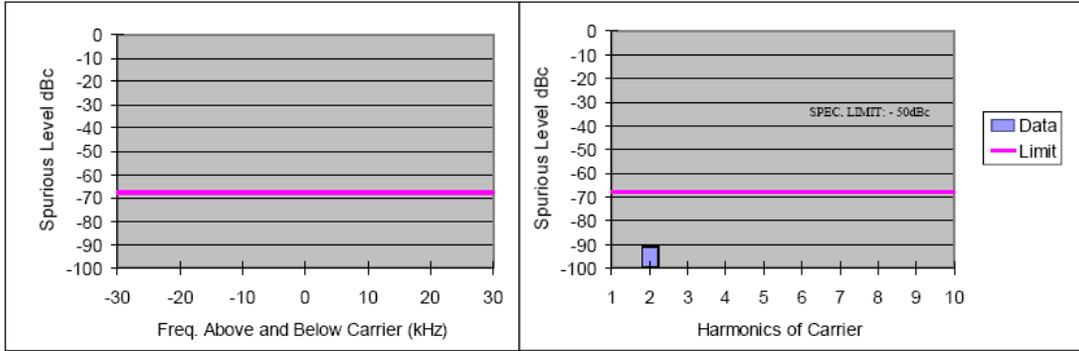
Figure 6G-25: 60 Watts Harmonic of Carrier 136.0125 MHz, 12.5 KHz Channel Spacing
