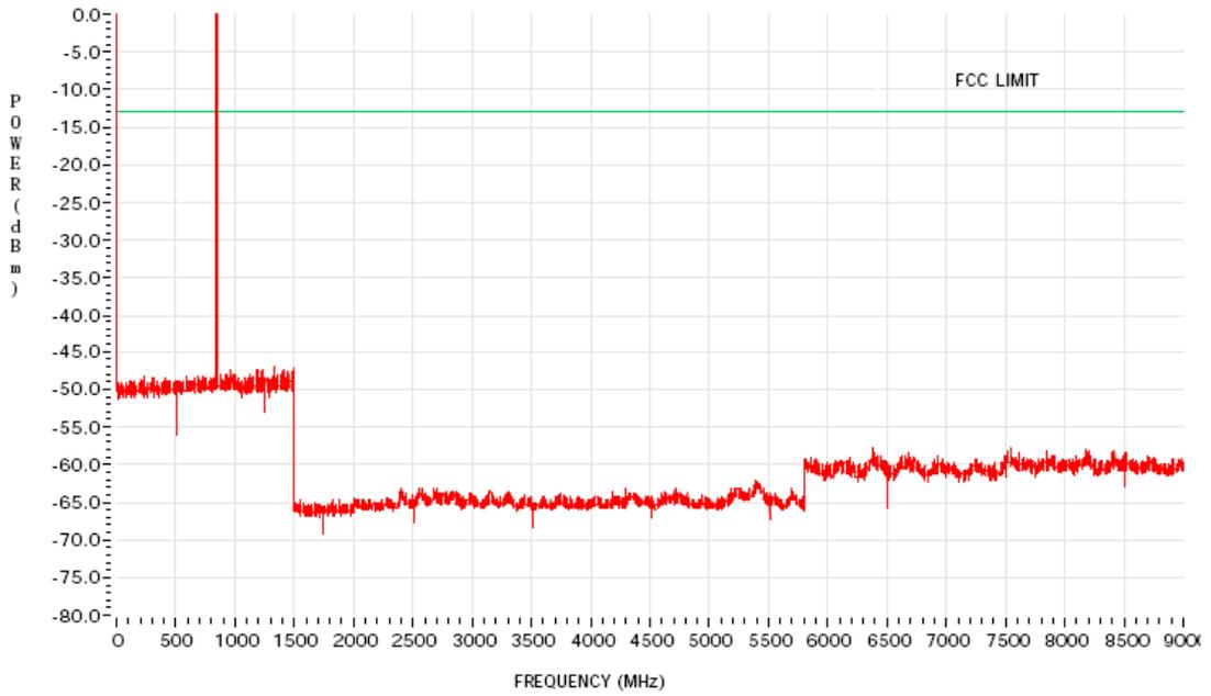
Figure 6G-21: 42 Watts Harmonic of Carrier 868.8875 MHz
