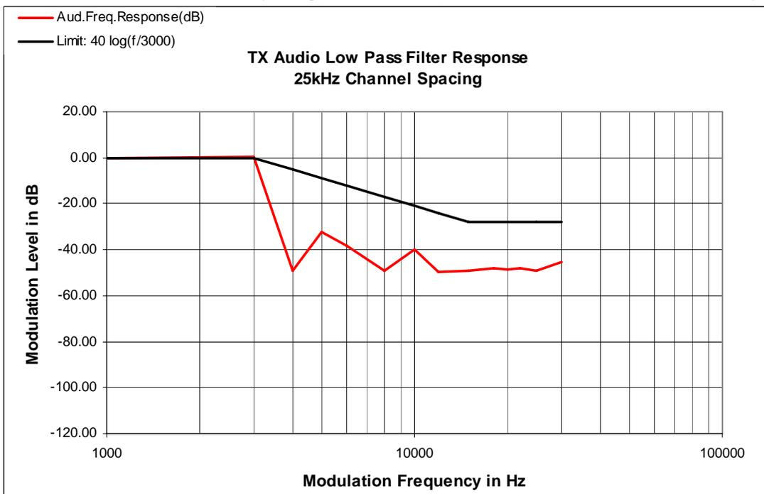
**Figure 6C-2:** 25 KHz Channel Spacing, 155.025 MHz, Transmit Audio Low Pass Filter Response
