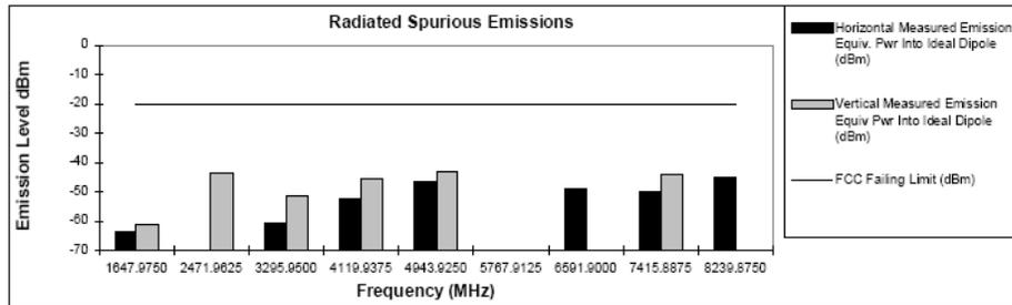
Figure 6H-21: 42 Watts, 823.9875MHz, 12.5 KHz Channel Spacing
