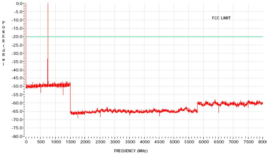
Figure 6G-28: 2 Watts Harmonic of Carrier 764.0125 MHz
