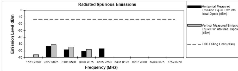
Figure 6H-7: 36 Watts, 775.9875MHz, 25 KHz Channel Spacing
