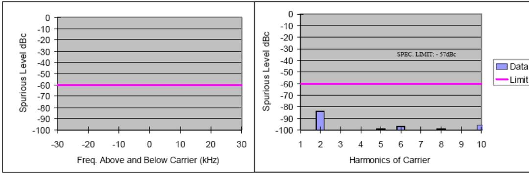
Figure 6G-33: 11 Watts Harmonic of Carrier 136.0125 MHz, 12.5 KHz Channel Spacing
