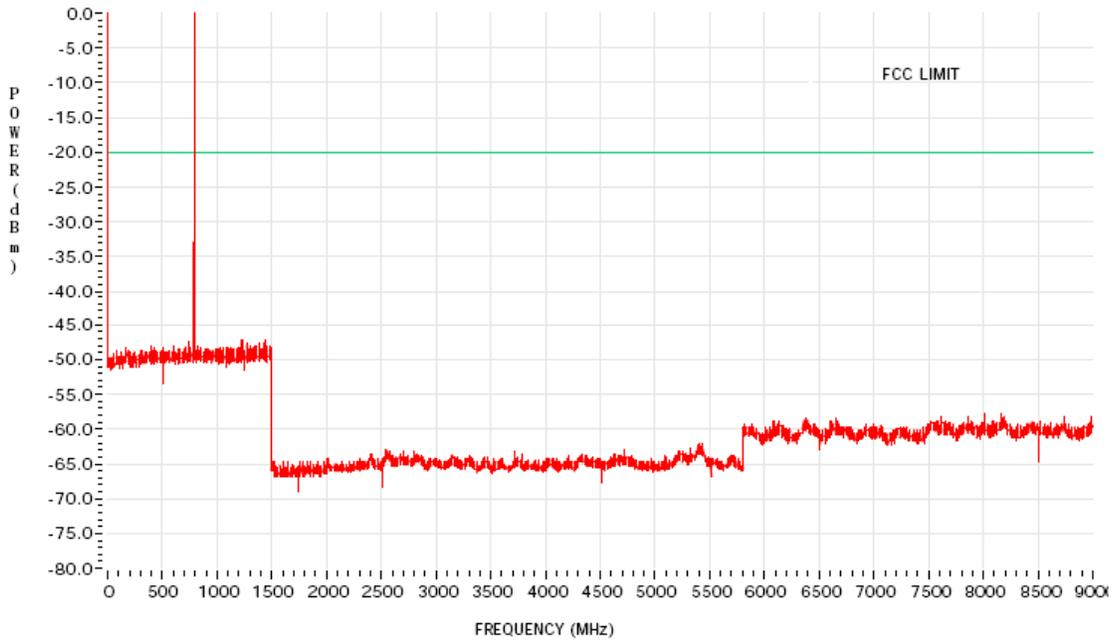
Figure 6G-30: 2 Watts Harmonic of Carrier 805.9875MHz
