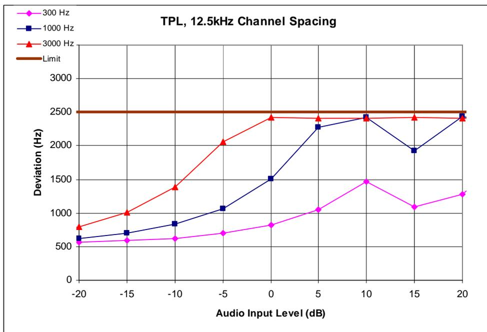
Figure 6D-2: 12.5 KHz Channel Spacing, 155.025 MHz, Tone Private Line (TPL) Mode
