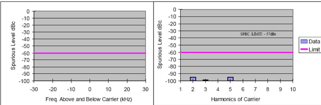
Figure 6G-24: 11 Watts Harmonic of Carrier 173.9875 MHz, 12.5 KHz Channel Spacing
