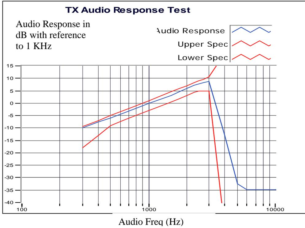
Figure 6B-4: 25 KHz Channel Spacing, 860.0125MHz, Transmit Audio Frequency Response
