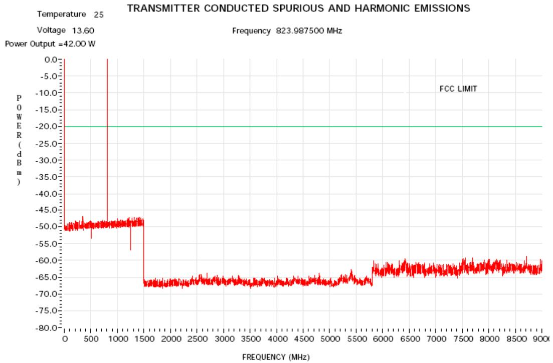
Figure 6G-28: 42 Watts Harmonic of Carrier 823.9875 MHz
