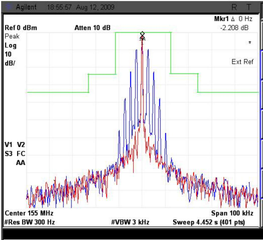
Figure 6E-3: 25KHz Channel Spacing, 155.0125 MHz, Analog Voice, Mask B 16K0F3E
