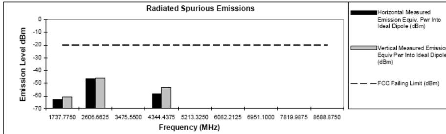
Figure 6H-17: 42 Watts, 868.887575MHz, 12.5 KHz Channel Spacing
