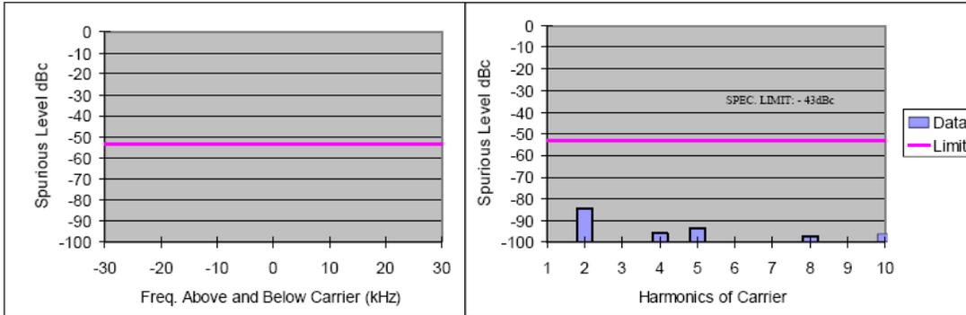
Figure 6I-7: 11 Watt Harmonic of Carrier 136.025 MHz, 25 KHz Channel Spacing
