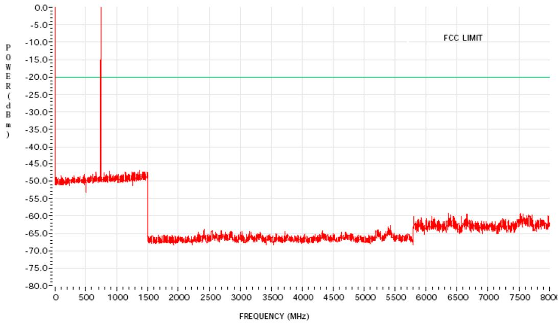
Figure 6G-39: 2 Watts Harmonic of Carrier 764.0125 MHz
