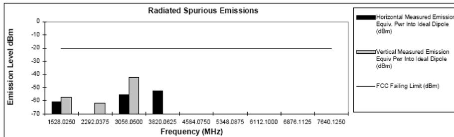
Figure 6H-18: 42 Watts, 764.0125MHz, 12.5 KHz Channel Spacing
