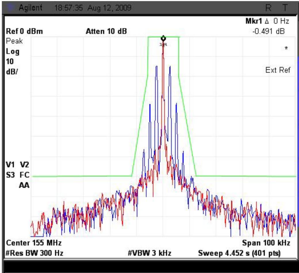
Figure 6E-1: 12.5 KHz Channel Spacing, 155.0125 MHz, Analog Voice, 11K0F3E
