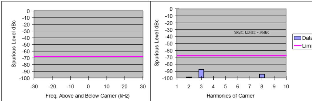
Figure 6G-38: 60 Watts Harmonic of Carrier 173.9875 MHz, 12.5 KHz Channel Spacing
