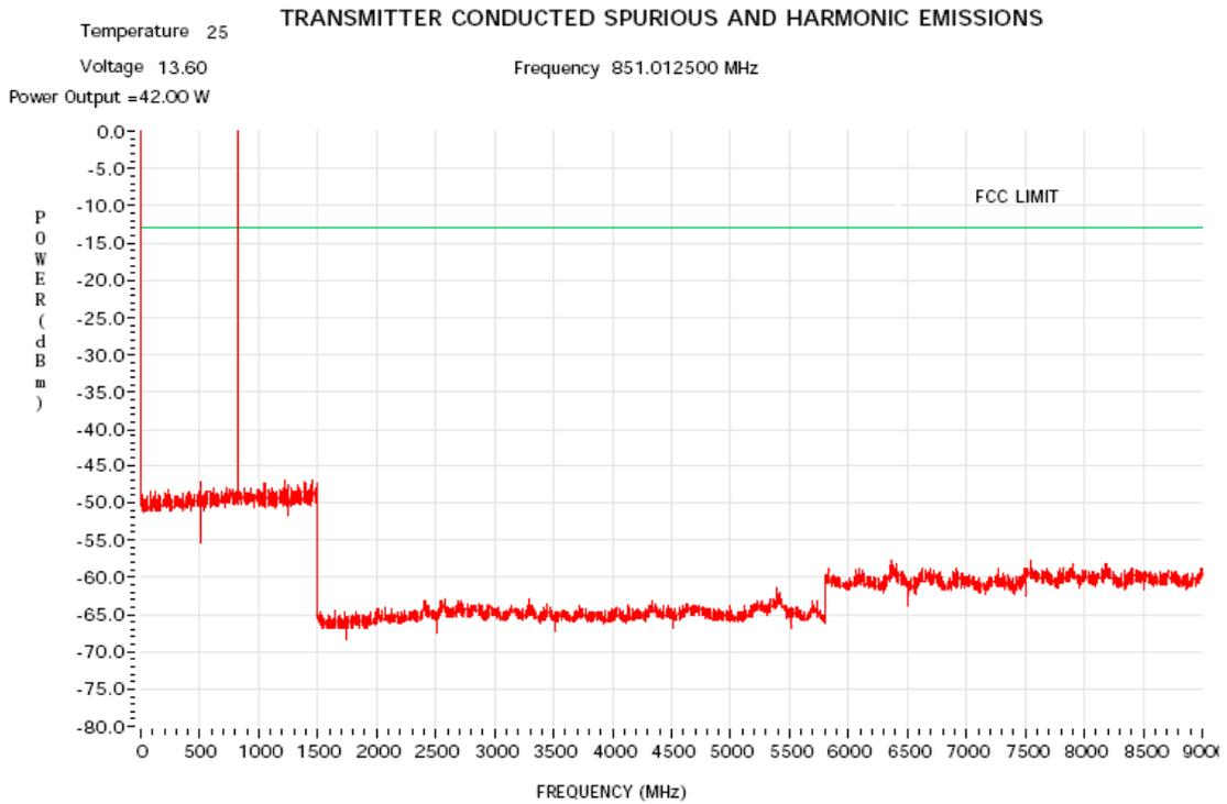
Figure 6G-20: 42 Watts Harmonic of Carrier 851.0125 MHz
