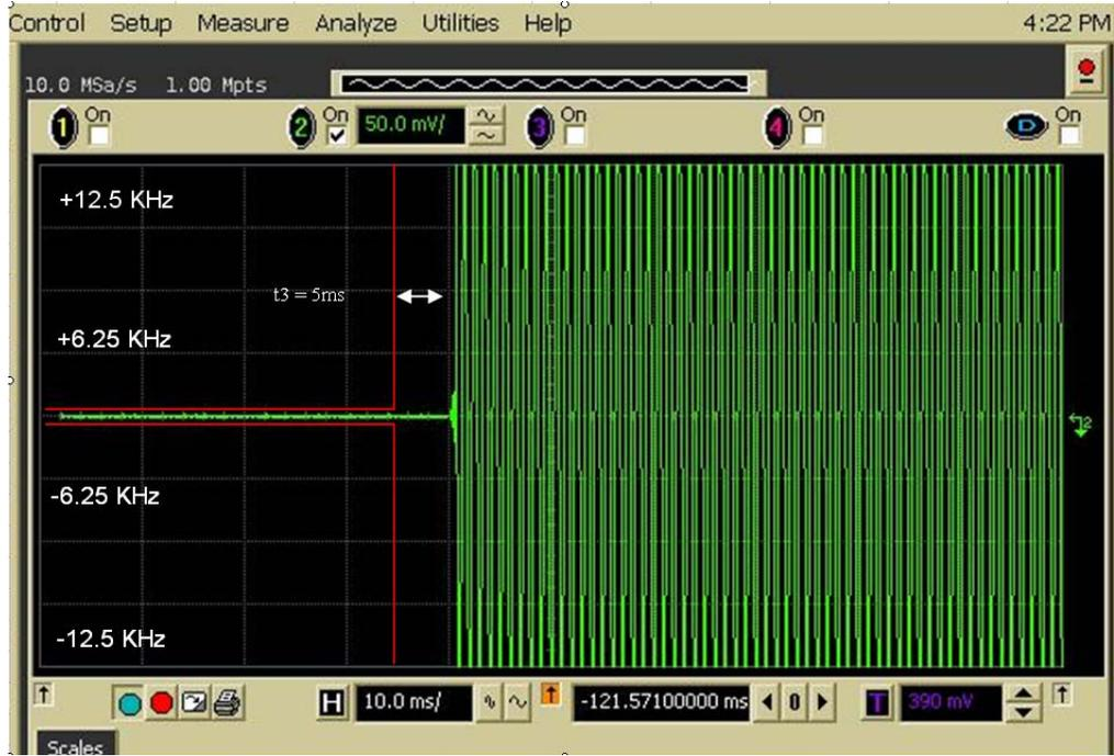
Figure 6K-4: Transient Frequency Behavior, 155.0125MHz, 12.5 KHz Channel Spacing, De-Key Transient
