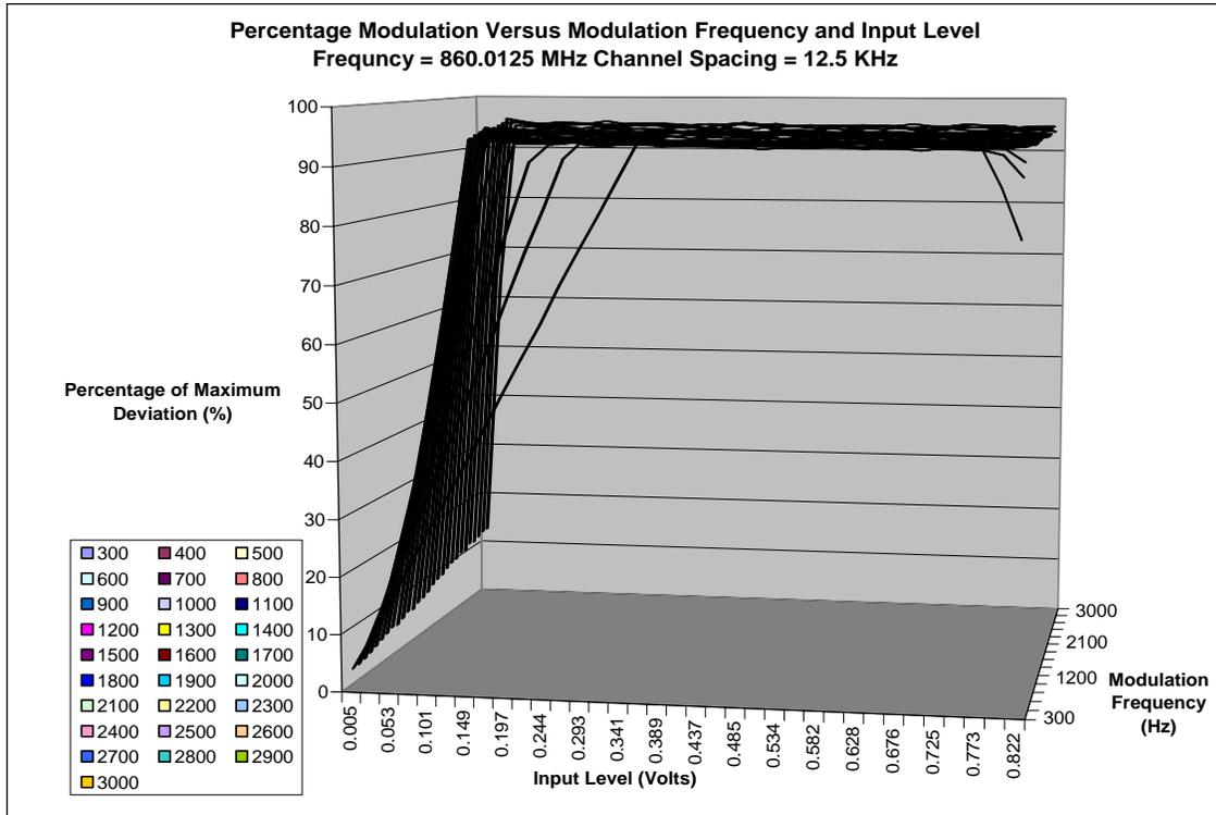
Figure 6D-7: The Percentage of Max. Deviation on the “Z” axis is referenced to 2.5 kHz for 12.5 kHz bandwidth
