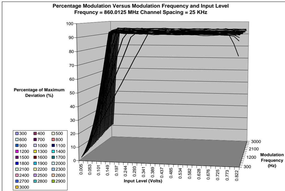
Figure 6D-8: The Percentage of Max. Deviation on the “Z” axis is referenced to 5.0 kHz for 25 kHz bandwidth
