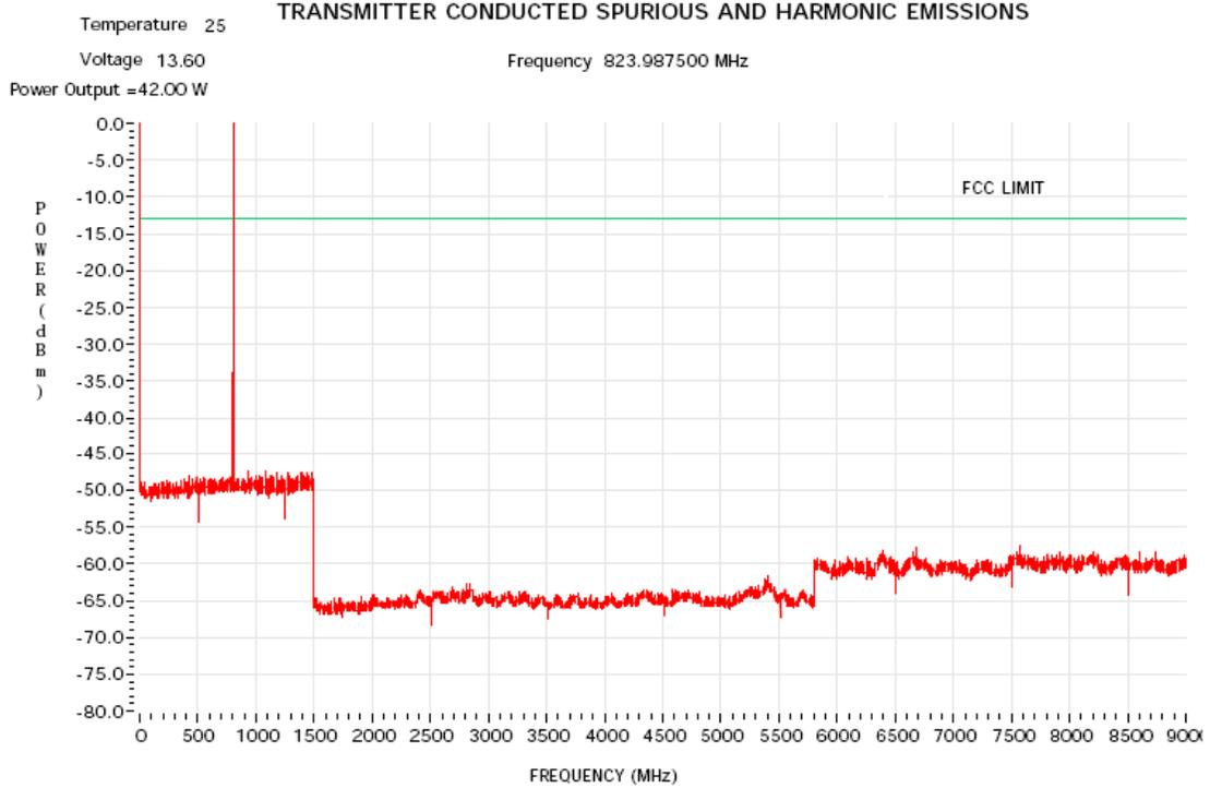
Figure 6G-19: 42 Watts Harmonic of Carrier 823.9875 MHz
