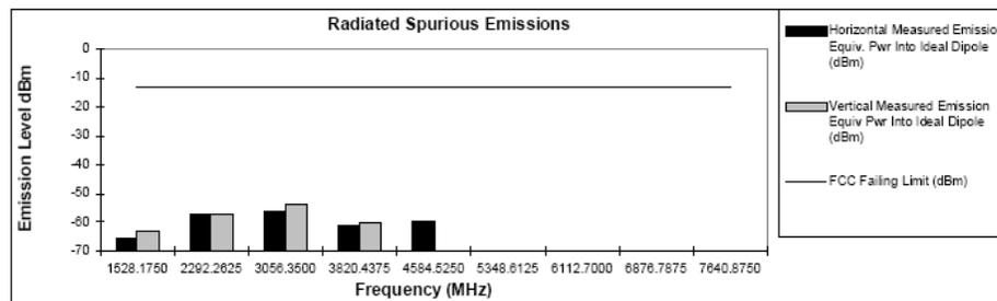
**Figure 6H-6: 36 Watts, 764.0875MHz, 25 KHz Channel Spacing**
