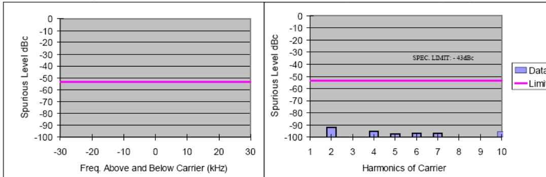
Figure 6G-9: 11 Watt Harmonic of Carrier 173.975 MHz, 25 KHz Channel Spacing
