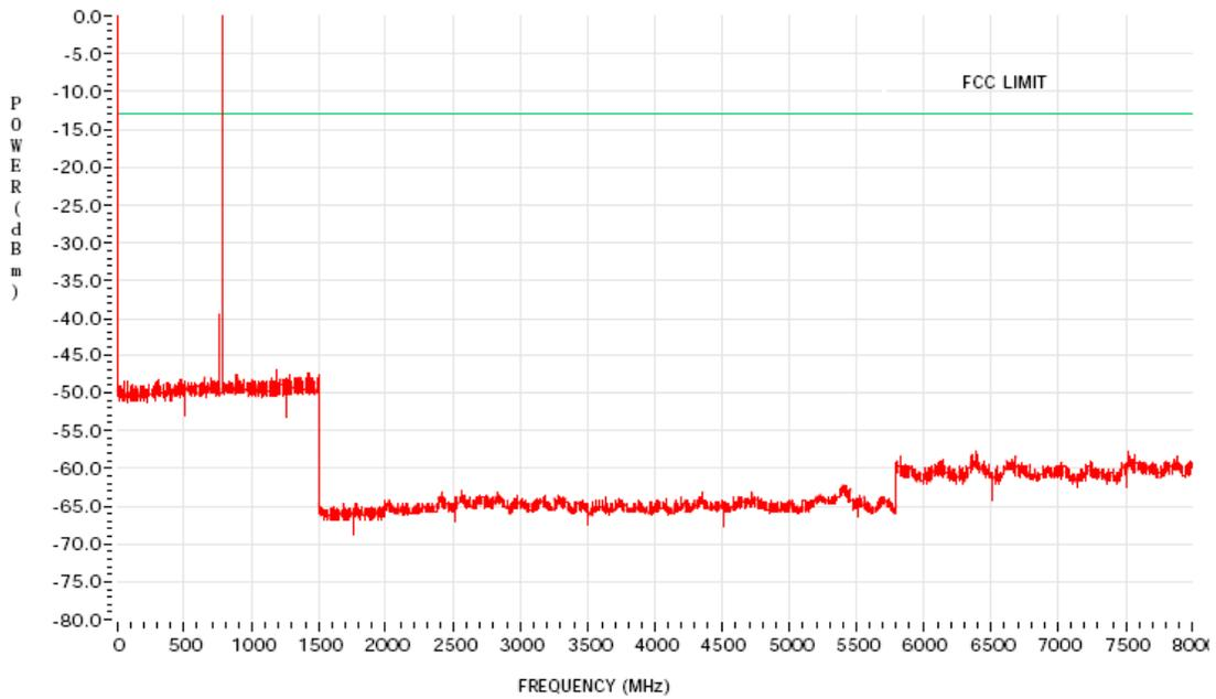
Figure 6G-16: 36 Watts Harmonic of Carrier 764.0125 MHz
