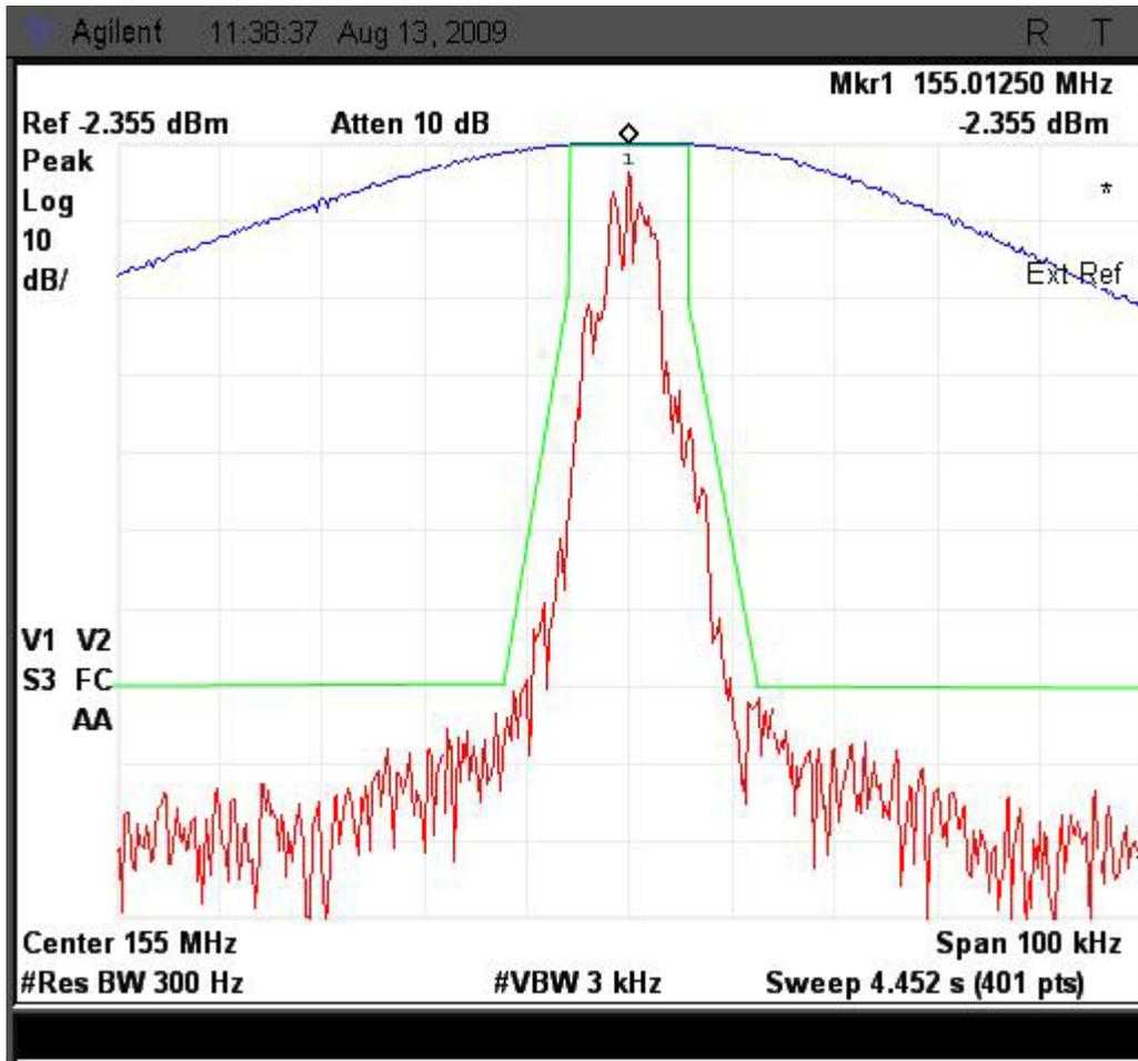
Figure 6F-13: 12.5 KHz Channel Spacing, 155.0125 MHz, Digital Voice Encryption Mask D 8K10F1E
