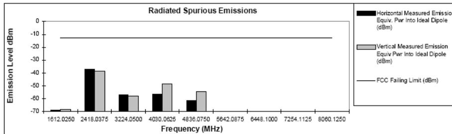
Figure 6H-10: 42 Watts, 806.0125MHz, 25 KHz Channel Spacing
