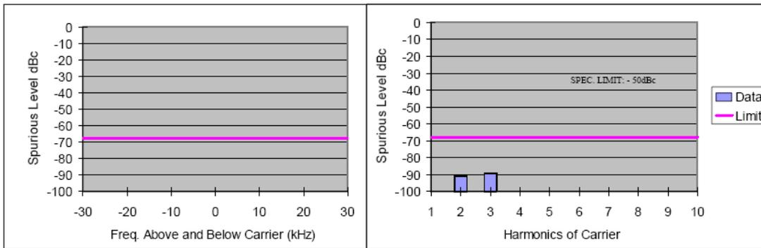
Figure 6G-11: 60 Watts Harmonic of Carrier 155.025 MHz, 25 KHz Channel Spacing
