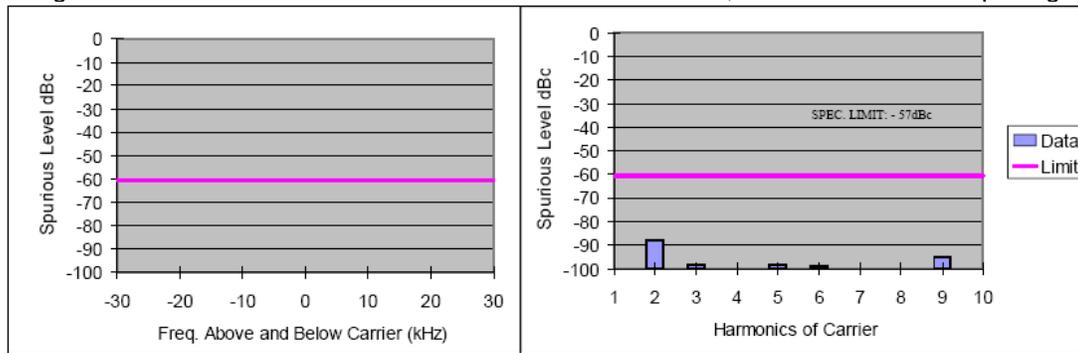
Figure 6G-34: 11 Watts Harmonic of Carrier 155.0125 MHz, 12.5 KHz Channel Spacing
