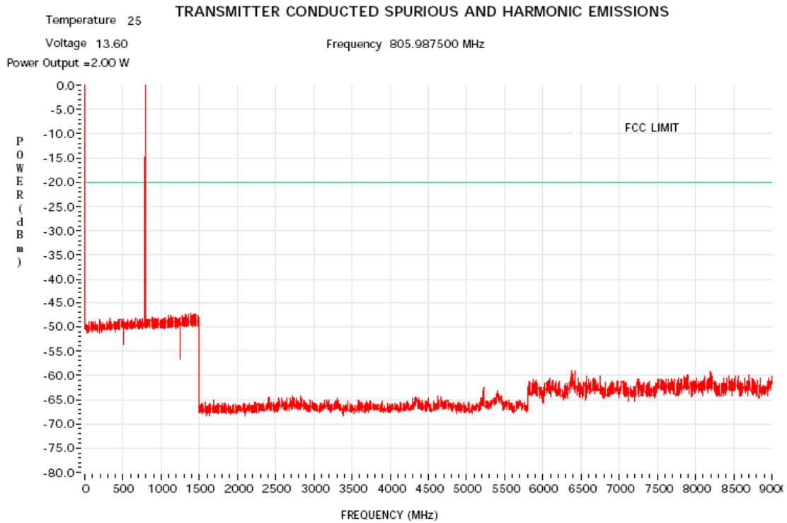
Figure 6G-41: 2 Watts Harmonic of Carrier 805.9875 MHz
