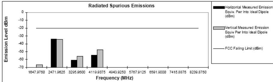
**Figure 6H-16: 42 Watts, 823.9875MHz, 12.5 KHz Channel Spacing**
