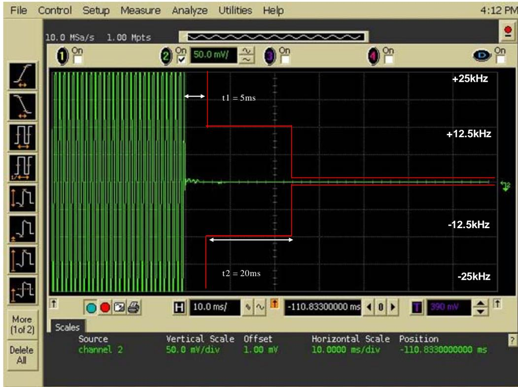
Figure 6K-1: Transient Frequency Behavior, 155.0125MHz, 25 KHz Channel Spacing, Key up Transient
