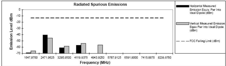
Figure 6H-11: 42 Watts, 823.9875MHz, 25 KHz Channel Spacing
