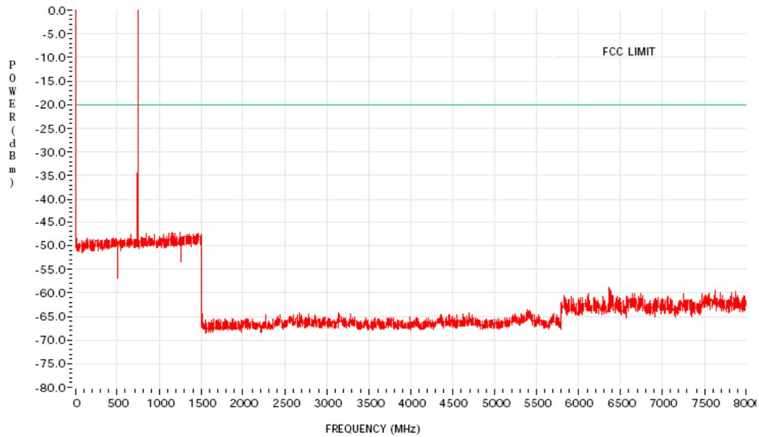
Figure 6G-40: 36 Watts Harmonic of Carrier 764.0875 MHz
