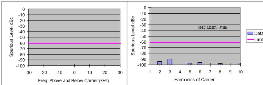
Figure 6G-35: 11 Watts Harmonic of Carrier 173.9875 MHz, 12.5 KHz Channel Spacing
