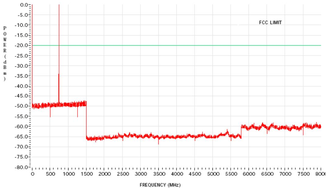
Figure 6G-29: 36 Watts Harmonic of Carrier 764.0875 MHz
