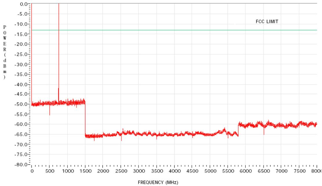
Figure 6G-15: 36 Watts Harmonic of Carrier 775.9875 MHz
