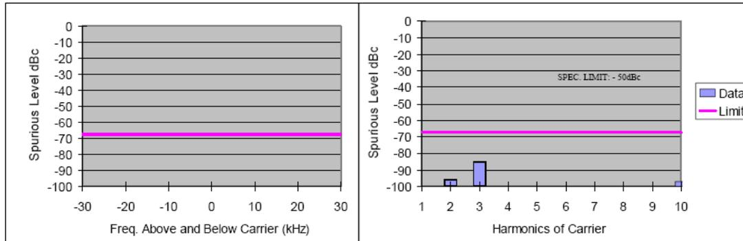
Figure 6G-12: 60 Watts Harmonic of Carrier 173.975 MHz, 25 KHz Channel Spacing
