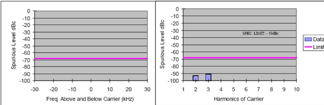
Figure 6G-26: 60Watts Harmonic of Carrier 155.0125 MHz, 12.5 KHz Channel Spacing
