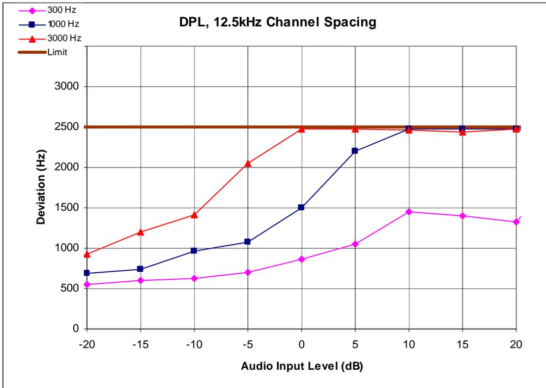
Figure 6D-3: 12.5 KHz Channel Spacing, 155.025 MHz, Digital Private Line (DPL) Mode
