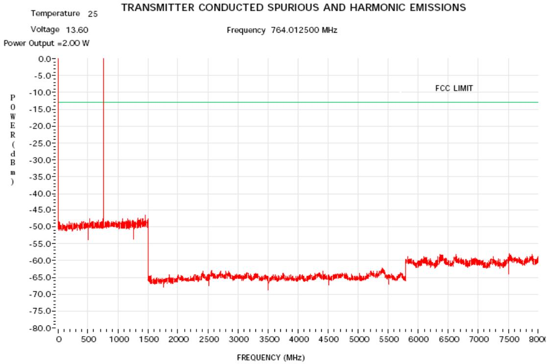
Figure 6G-13: 2 Watts Harmonic of Carrier 764.0125 MHz
