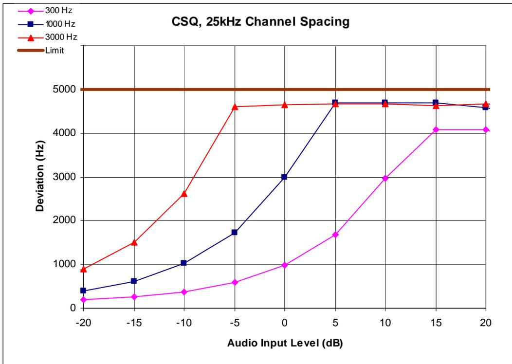
Figure 6D-4: 25 KHz Channel Spacing, 155.025 MHz, Carrier Squelch (CSQ) Mode
