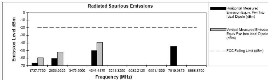
Figure 6H-22: 42 Watts, 868.8875MHz, 12.5 KHz Channel Spacing
