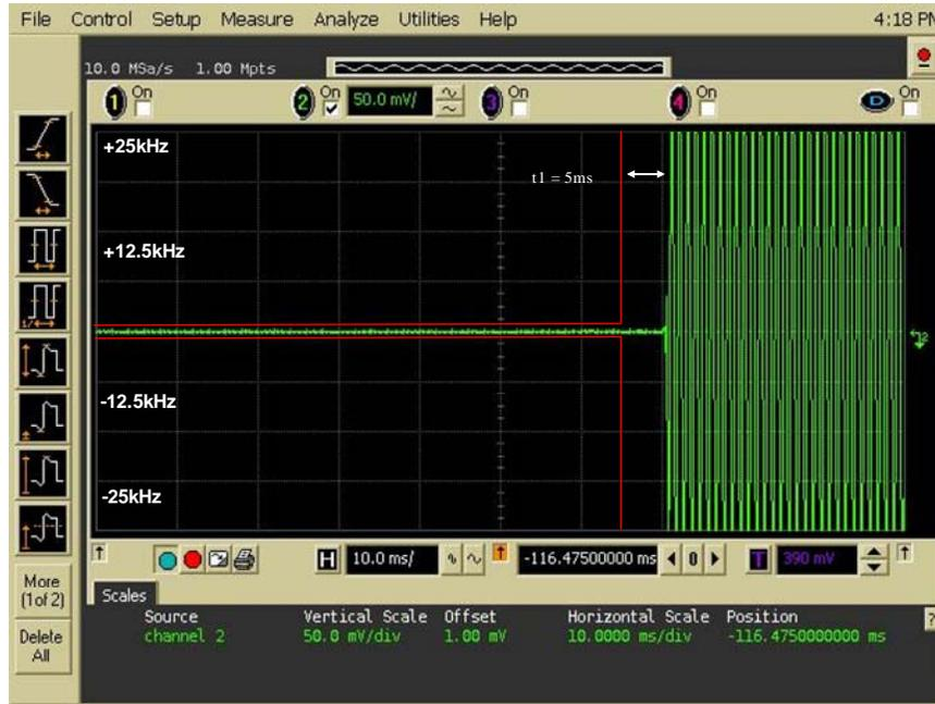
Figure 6K-2: Transient Frequency Behavior, 155.0125MHz, 25 KHz Channel Spacing, De- Key Transient
