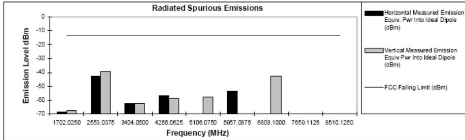
Figure 6H-12: 42 Watts, 851.0125MHz, 25 KHz Channel Spacing
