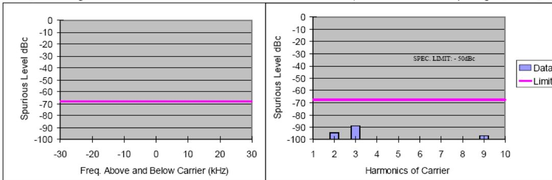
Figure 6G-37: 60Watts Harmonic of Carrier 155.0125 MHz, 12.5 KHz Channel Spacing
