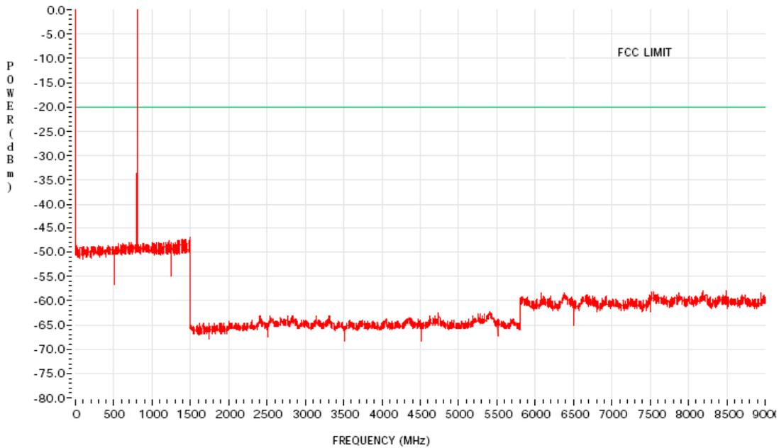
Figure 6G-31: 42 Watts Harmonic of Carrier 823.9875 MHz
