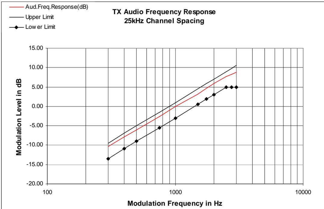
Figure 6B-2: 25 KHz Channel Spacing, 155.0125 MHz, Transmit Audio Frequency Response
