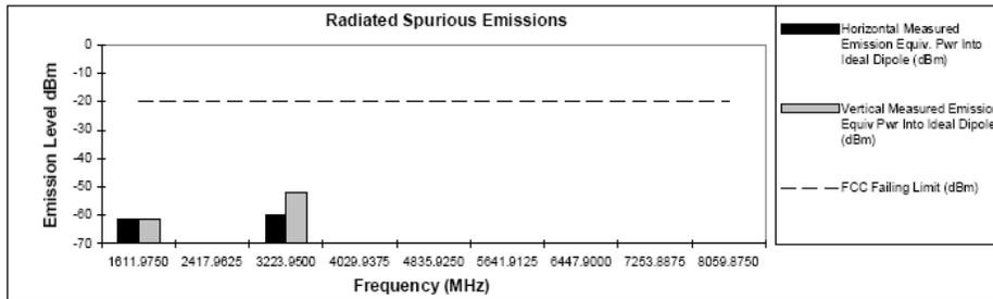
Figure 6H-20: 2 Watts, 805.9875MHz, 12.5 KHz Channel Spacing
