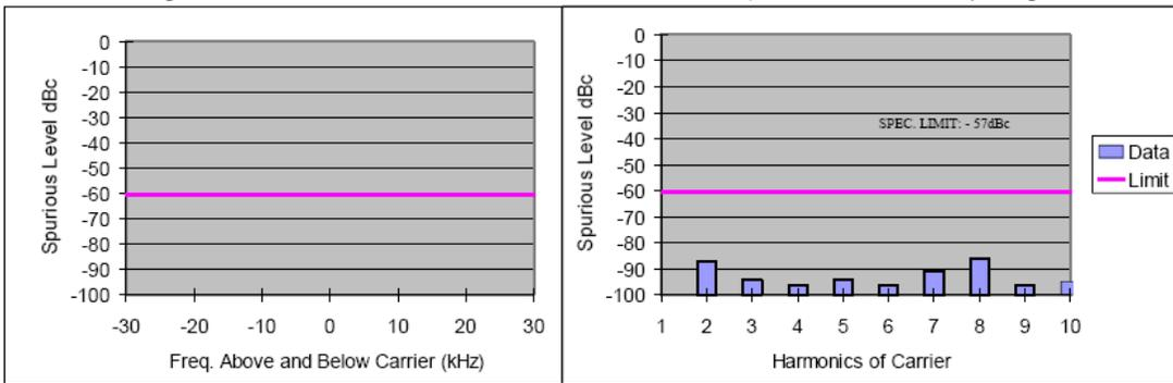
Figure 6G-23: 11 Watts Harmonic of Carrier 155.0125 MHz, 12.5 KHz Channel Spacing
