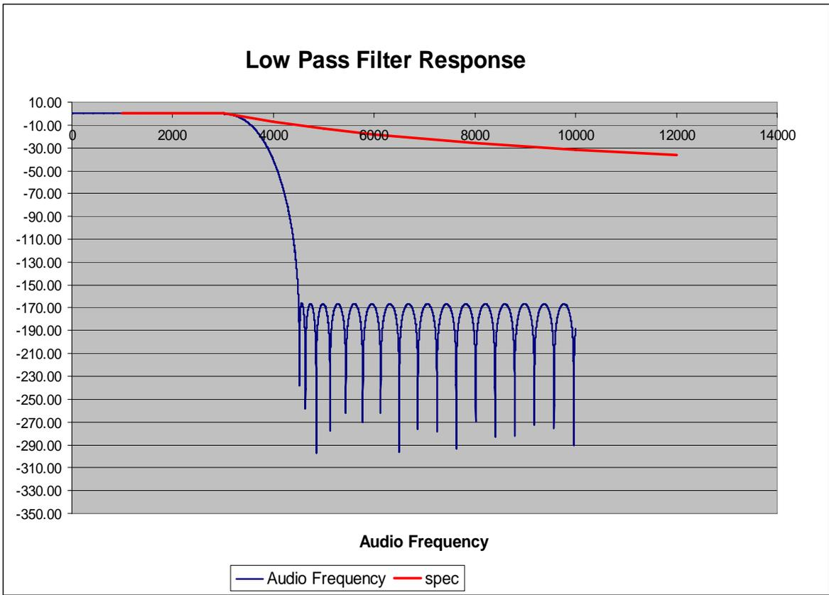
Figure 6C-3: 156.0125MHz, Transmit Audio Low Pass Filter Response
