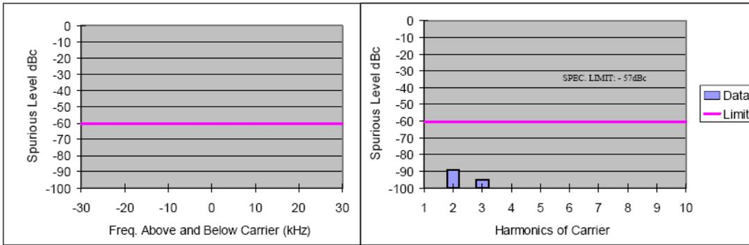
Figure 6G-22: 11 Watts Harmonic of Carrier 136.0125 MHz, 12.5 KHz Channel Spacing
