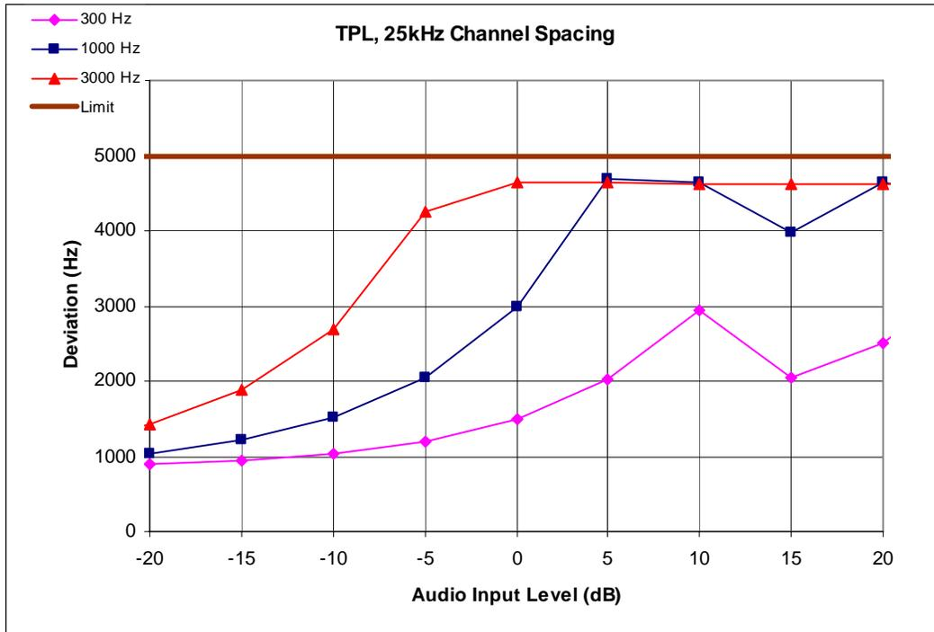
Figure 6D-5: 25 KHz Channel Spacing, 155.025 MHz, Tone Private Line (TPL) Mode
