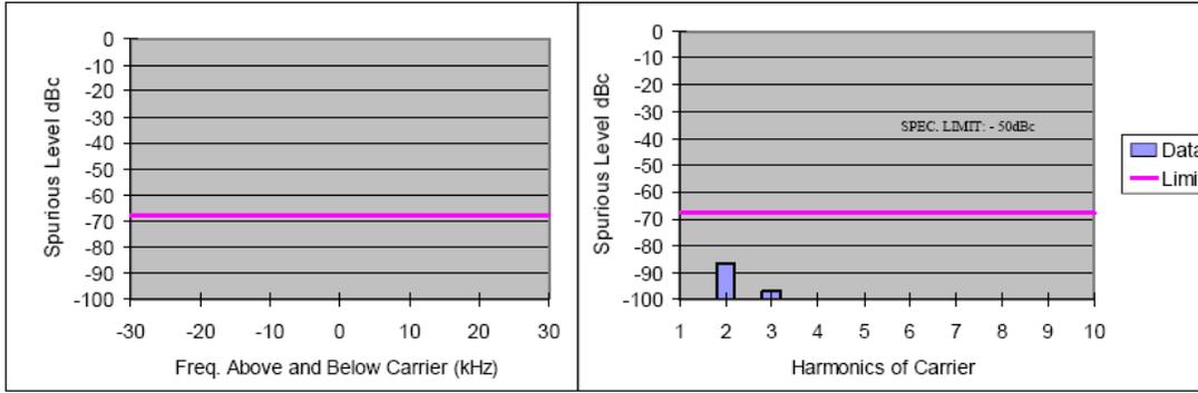
Figure 6G-10: 60 Watts Harmonic of Carrier 136.025 MHz, 25 KHz Channel Spacing
