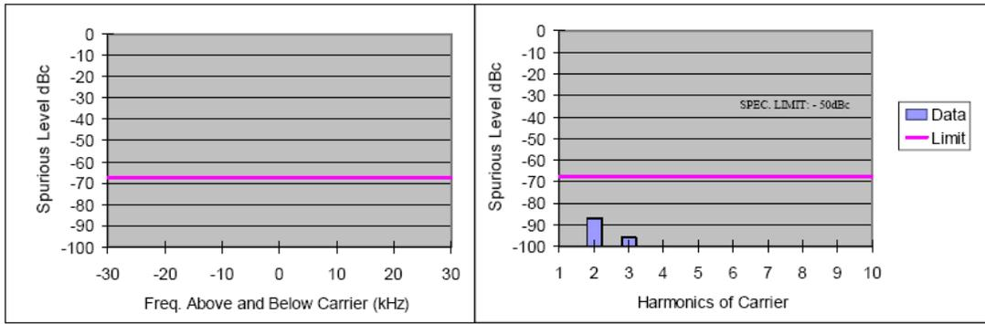
Figure 6G-36: 60 Watts Harmonic of Carrier 136.0125 MHz, 12.5 KHz Channel Spacing
