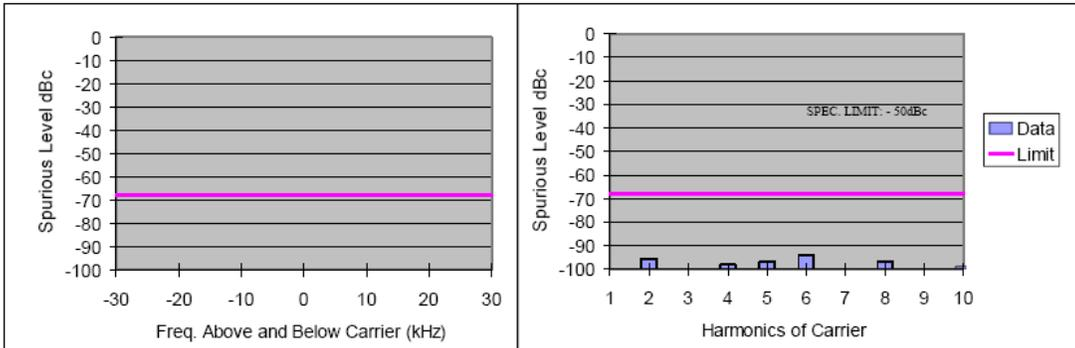
Figure 6G-27: 60 Watts Harmonic of Carrier 173.9875 MHz, 12.5 KHz Channel Spacing
