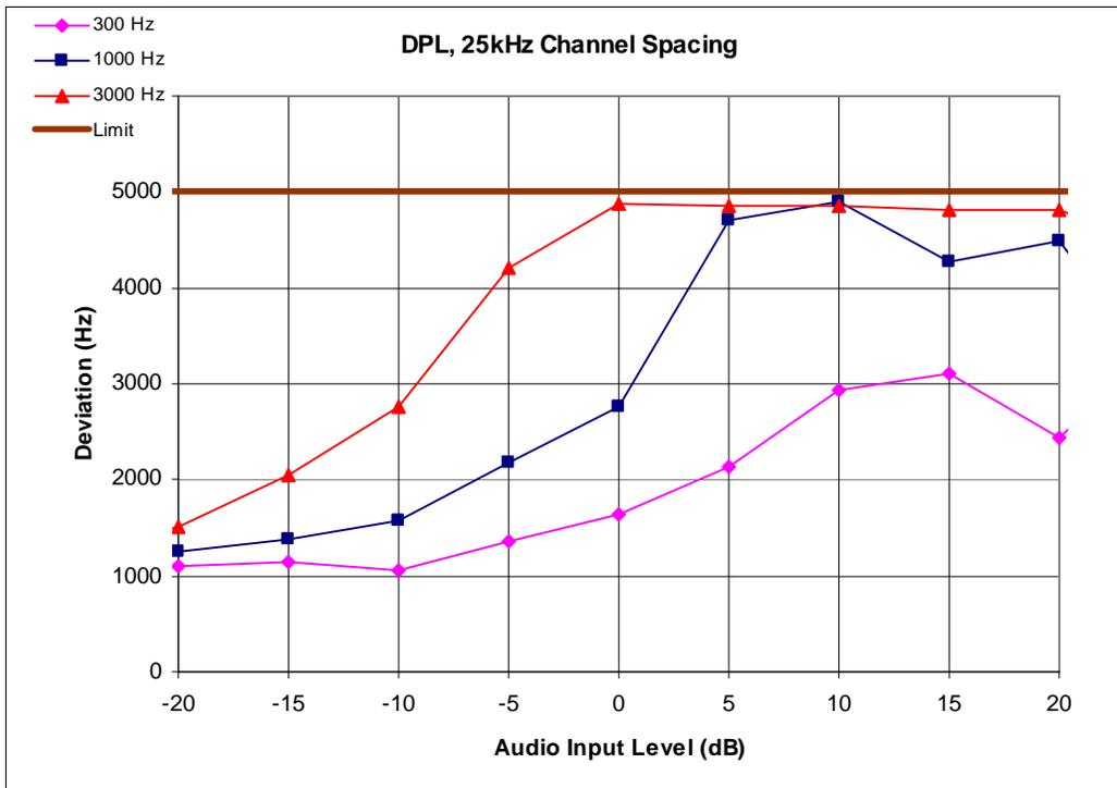
Figure 6D-6: 25 KHz Channel Spacing, 155.025 MHz, Digital Private Line (DPL) Mode
