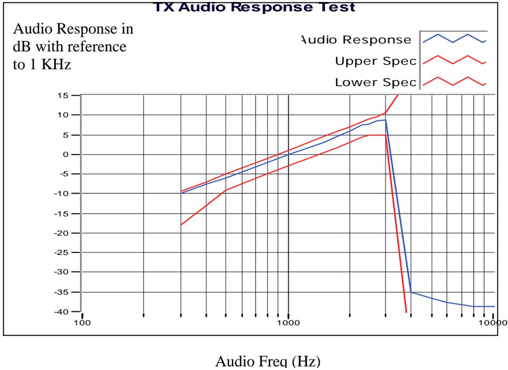
Figure 6B-3: 12.5 KHz Channel Spacing, 860.0125MHz, Transmit Audio Frequency Response
