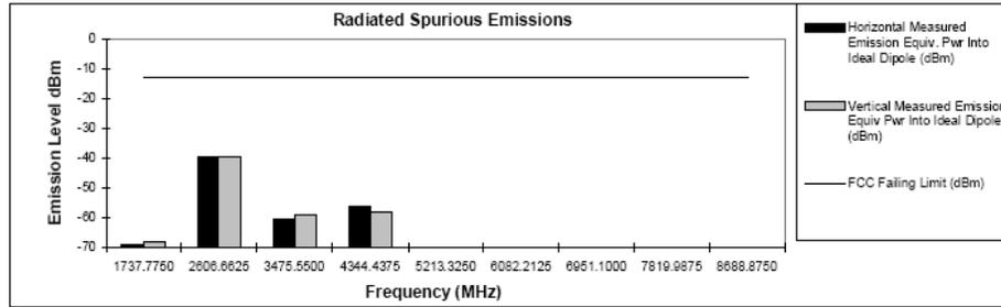
Figure 6H-13: 42 Watts, 868.8875MHz, 25 KHz Channel Spacing
