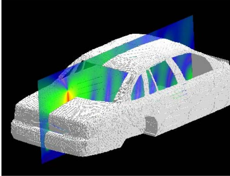
The equivalent power density (S) is computed from the E-field and the H-field separately. The following table reports the E-field values computed by XFDTD™ at the six locations, and the corresponding power density.
