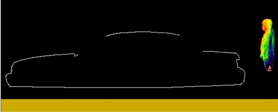
**Figure 7. SAR distribution at 174 MHz in the bystander located at back the trunk, produced by the trunk-mount RAD4010ARB antenna. The contour plot for SAR distribution in the figure is relative to the plane where the peak 1-g average SAR for this exposure condition occurs.**
