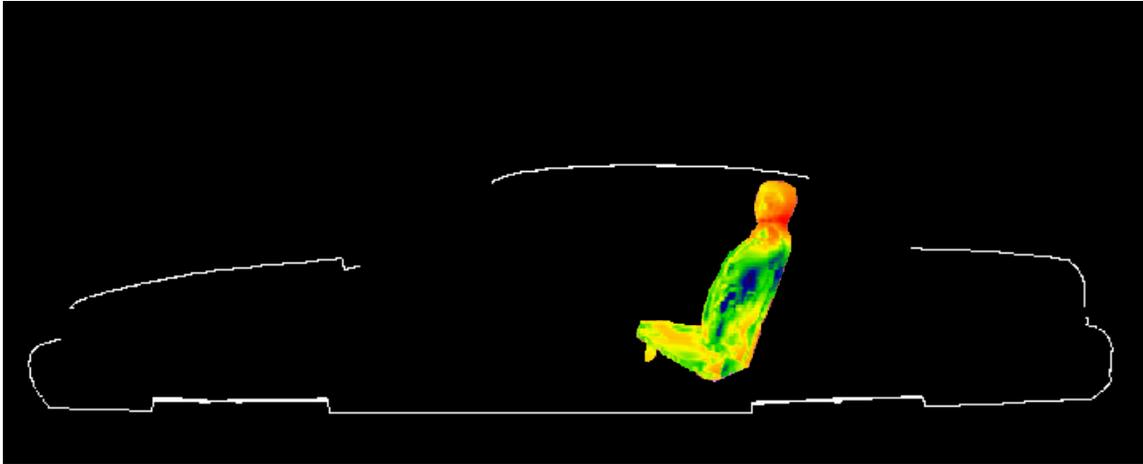
**Figure 4. SAR distribution at 174 MHz in the passenger located on the side of the back seat, produced by the trunk-mount RAD4010ARB antenna (103.5 cm). The contour plot in the figure is relative to the plane where the peak 1-g average SAR for this exposure condition occurs.**
