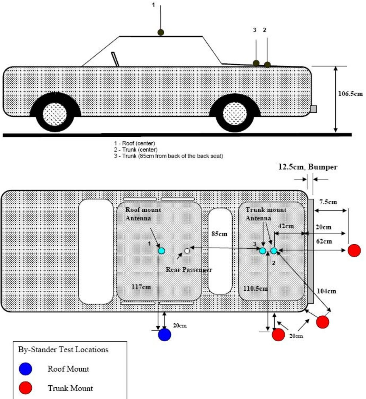
Figure 2: Illustration of Antenna Locations and Test Distances for the assessment at VHF Band
