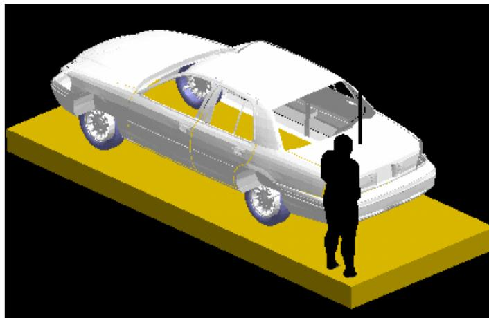
**Figure 1: Bystander model exposed to a trunk-mount VHF antenna: Bystander is located at the back, on the side or at the corner of the car replicating the measurement conditions. The antenna is mounted in the center of the trunk. The dielectric slab under the car is introduced to model the ground (pavement) effect on exposure.**
