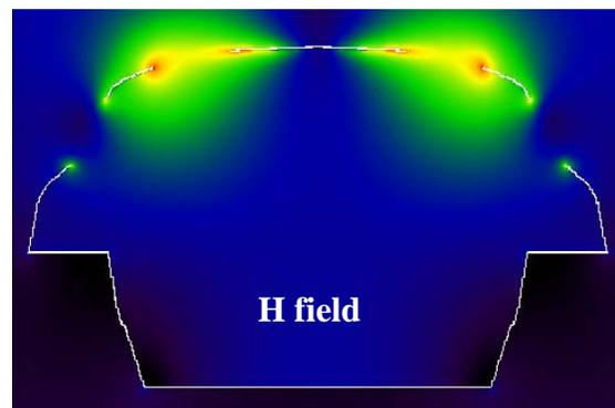
The highest exposure occurs in the middle of the backseat, which is also the case in the measurements. Therefore, the field values were determined on the yellow line centered at the middle of the backseat, approximately at the three locations that are shown by white dots. In actuality, the line is inclined so as to follow the inclination of the passenger's
