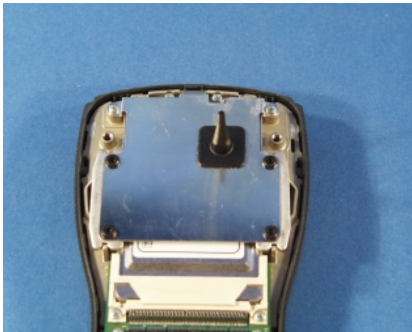
Antenna Photograph Installed
