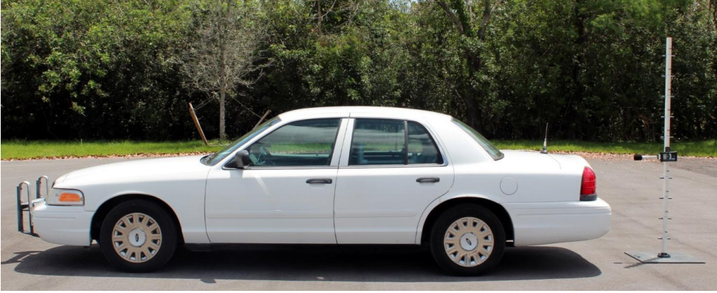
Test measurement setup for Bystander, trunk mount antenna behind vehicle
